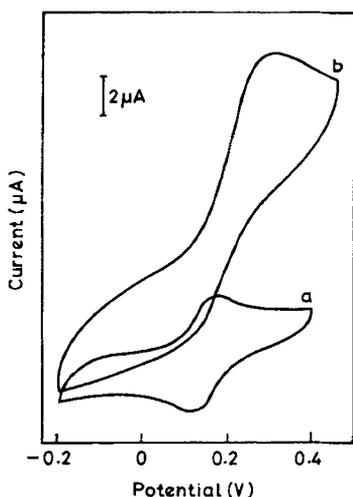
**Figure 1.** Cyclic voltammograms of (a) BQ/GOD modified electrode, (b) as in (a) with 20 mM glucose solution. Scan speed: 5 mV/s in 0.2 M phosphate buffer (pH 7.1)
