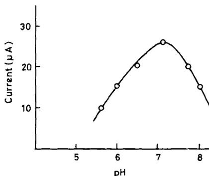
**Figure 5.** pH profile of the BQ/GOD modified electrode with 20 mM glucose. Scan speed: 10 mV/s in 0.2 M phosphate buffer (pH 7.1).
