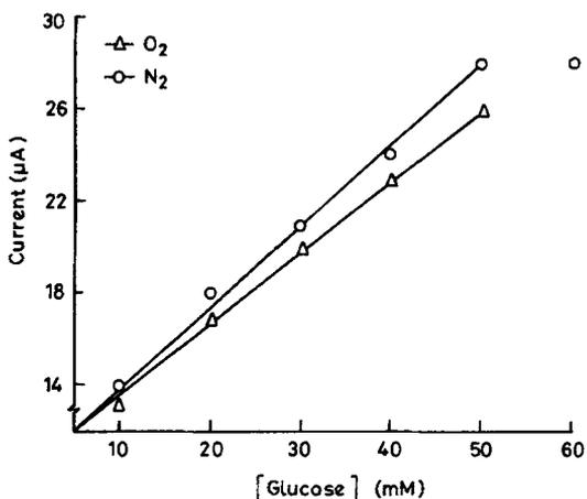
**Figure 3.** Calibration curves for the GOD modified electrode poised at 0.25 V vs Ag/AgCl in (○) N<sub>2</sub> saturated and (Δ) O<sub>2</sub> saturated phosphate buffer (pH 7.1). Scan speed: 5 mV/s.
