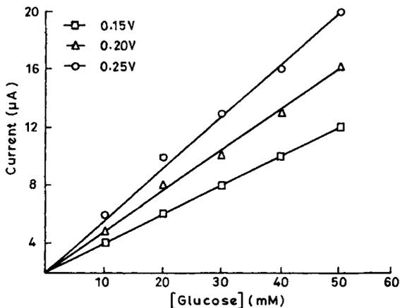
**Figure 2.** Effect of operating potential on the response to glucose. (□) 0.15 V, (Δ) 0.20 V and (○) 0.25 V vs. Ag/AgCl. Scan speed: 5 mV/s in 0.2 M phosphate buffer (pH 7.1).
