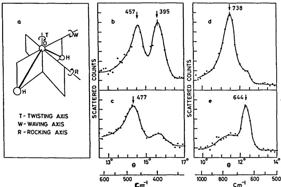
**Figure 4.** (a) Librational modes of water molecule. Neutron inelastic scattering spectra from single crystals of (b) and (c)  $\text{Ba}(\text{ClO}_3)_2 \cdot \text{H}_2\text{O}$ , and (d) and (e)  $\text{K}_2\text{Cl}_2\text{O}_4 \cdot \text{H}_2\text{O}$  at 120 K. All measurements are with the water molecule perpendicular to the scattering plane. (b) and (d) for twisting and waving motion and (c) and (e) for rocking motion.
