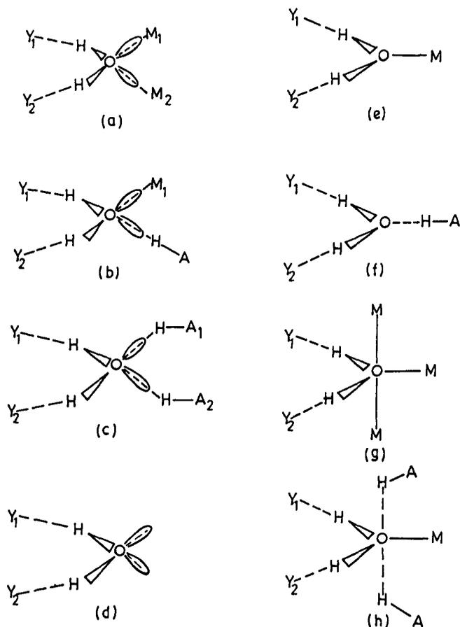
**Figure 1.** Classification of the lone-pair coordination of the water molecule deduced from neutron studies on crystal hydrates. (a, b, c) Tetrahedral coordinations with two lone-pairs pointing towards M or H atoms; (d) uncoordinated tetrahedral lone pairs; (e, f) trigonal coordinations; (g, h) trigonal bipyramidal coordinations.
