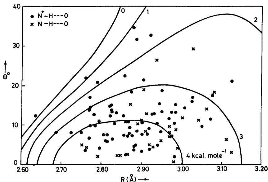
**Figure 5.** Equi-energy contours for N<sup>+</sup>-H...O hydrogen bonds in the  $R - \theta$  plane.  $R$  is the donor-acceptor distance and  $\theta$  is the bending angle at the donor atom. Experimentally observed positions of N<sup>+</sup>-H...O (●) and N-H...O (x) are also shown.
