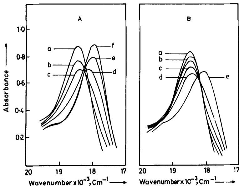
**Figure 1.** Absorption spectra of RB-BSA complex at pH 7.4 (A) and 12.7 (B). Spectra in  $20.0 \mu\text{M}$  of RB only (a), and in presence of BSA (b)-(f). [BSA] (in  $\mu\text{M}$ ) in (A) = 0.5(b), 1.0 (c), 2.0 (d), 4.0 (e), 20.0 (f) and in (B) = 0.5 (b), 2.0 (c), 4.0 (d), 20.0 (e).
