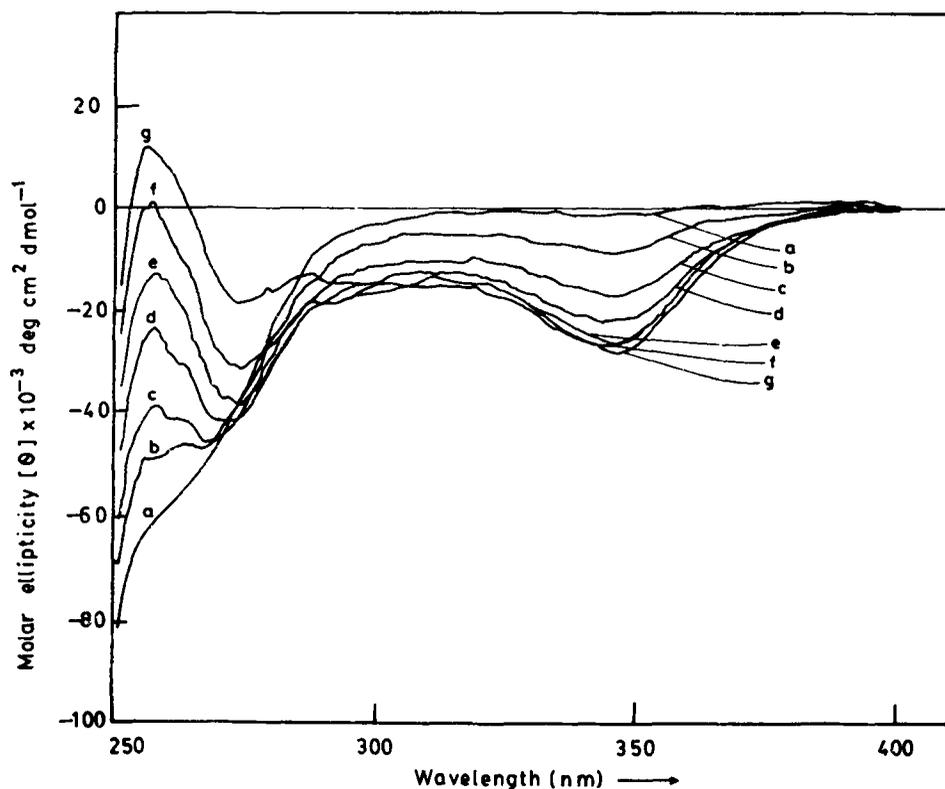
**Figure 3.** Circular dichroism spectra at pH 7.4 for RB-BSA interaction. (a) 20.0  $\mu\text{M}$  of BSA only. (b)–(g): BSA + RB. [RB] (in  $\mu\text{M}$ ) = 10.0 (b), 20.0 (c), 30.0 (d), 40.0 (e), 50.0 (f) and 70.0 (g).
