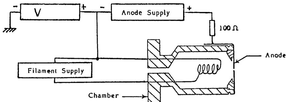
Figure 2. Schematic diagram of the high pressure plasma ion source.
