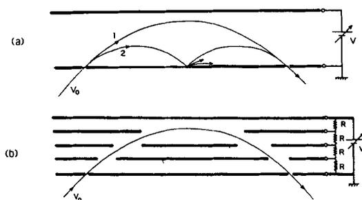
**Figure 5.** Schematic diagram of the parallel plate electrostatic energy analyser. (a) Two possible trajectories followed by low energy ions traversing the energy analyser. Trajectory 2 shows the occurrence of ion reflection from the copper surface of the lower analyser plate. (b) Inclusion of suitably biased intermediate plates eliminates the possibility of reflected ions being transmitted.
