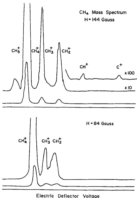
**Figure 4.** Mass spectrum of  $\text{CH}_4$  obtained under two different magnetic fields in the Wien filter.
