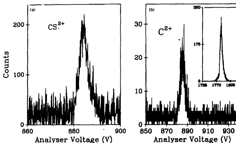
**Figure 6.** (a) Translational energy spectrum of metastable  $CS^{2+}$  ions resulting from the charge stripping reaction  $CS^+ \rightarrow CS^{2+}$ . (b) Translational energy spectrum of  $C^{2+}$  ions resulting from the charge stripping reaction  $C^+ \rightarrow C^{2+}$ . Inset shows the  $C^+$  peak which is elastically scattered in 3 keV collisions with He. This spectrum is used for calibrating the energy scale in (a).
