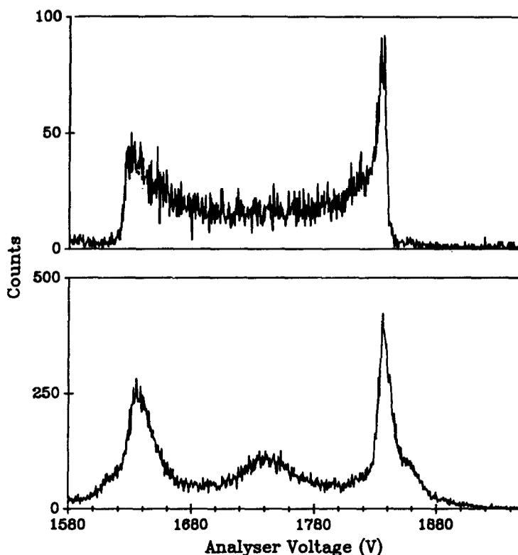
Figure 8. Translational energy spectrum of  $O^+$  fragments resulting from dissociation of metastable CO at He collision gas pressures of  $1 \times 10^{-6}$  Torr (upper panel) and  $1 \times 10^{-5}$  Torr (lower panel).
