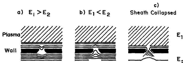
**Figure 3.** Ion extraction conditions as a function of applied extraction field  $E_2$  and the mean electric field within the ion source  $E_1$ . Our operating conditions induce the plasma sheath to collapse, as indicated in case (c).
