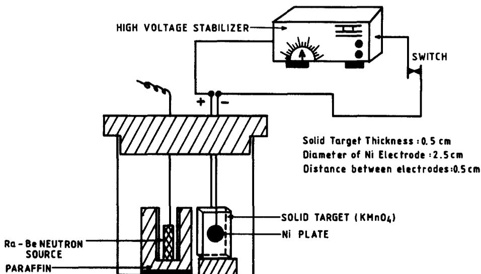
Figure 1. Arrangement for neutron activation and collection of  $(n, \gamma)$  recoil species ( $^{56}\text{Mn}^*$ ) of  $\text{KMnO}_4$  on nickel plates.
