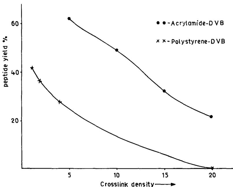
**Figure 2.** Effect of crosslink density on peptide yield for the synthesis of Boc-Gly-Phe-OMe using papain immobilized on polystyrene-DVB and polyacrylamide-DVB based supports.
