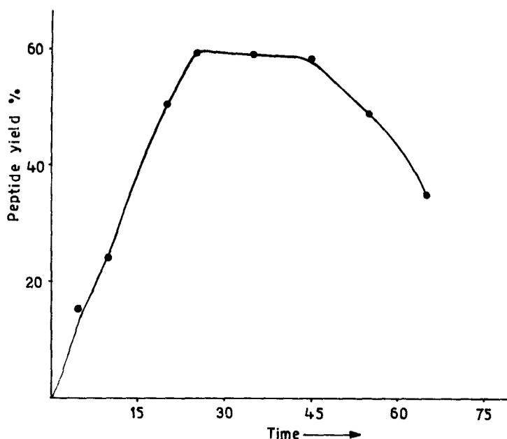
**Figure 4.** Effect of duration of reaction on peptide yield for the synthesis of Boc-Gly-Phe-OMe (concentration of Boc-Gly and Phe-OMe, 0.8 mmol each, immobilized papain 500 mg polymer  $\equiv$  20 mg of bound papain).
