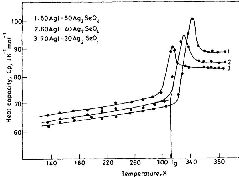
Figure 2. Variation of heat capacity with temperature for the glasses in the system AgI-Ag<sub>2</sub>SeO<sub>4</sub>.
