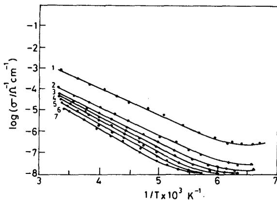
Figure 6. Variation of the a.c. conductivity with temperature at different frequencies for the glass  $50\text{AgI-}50\text{Ag}_2\text{SeO}_4$ . Numbers 1-7 correspond to frequencies (in kHz) 100, 30, 10, 3, 1, 0.3 and 0.1, respectively.
