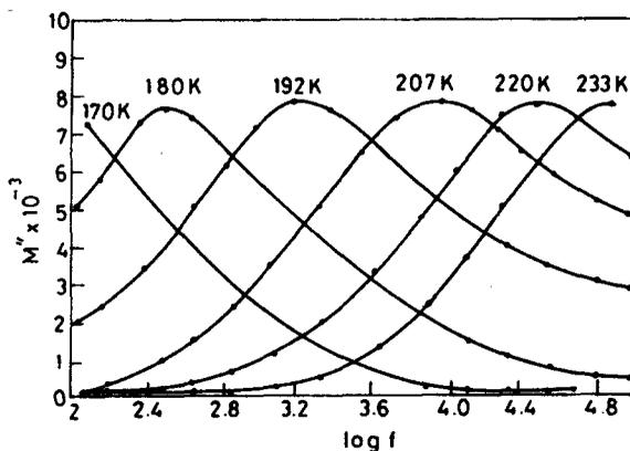
Figure 10. Variation of the imaginary part of the electric modulus ( $M''$ ) with frequency at different temperatures for the glass 50AgI-50Ag<sub>2</sub>SeO<sub>4</sub>.
