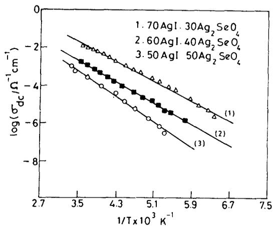
Figure 4. Variation of the d.c. conductivity with temperature for the glasses in the system  $\text{AgI-Ag}_2\text{SeO}_4$ .
