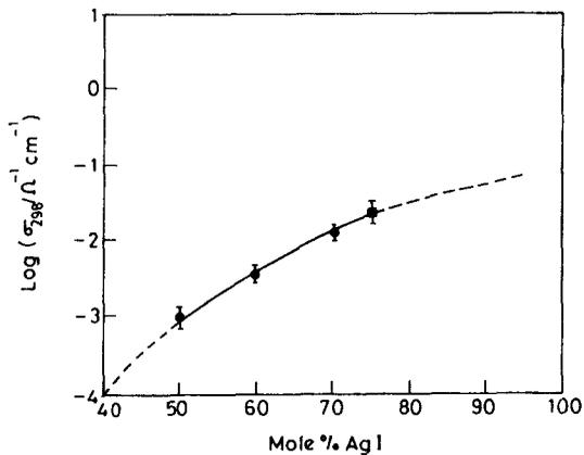
Figure 5. Variation of the conductivity at 298 K with mol% AgI for the glasses in the system  $\text{AgI-Ag}_2\text{SeO}_4$ .
