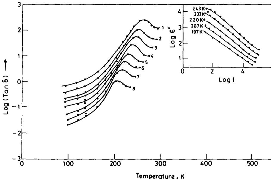
Figure 8. Variation of the loss angle with temperature for the glass 50AgI-50Ag<sub>2</sub>SeO<sub>4</sub>. Numbers 1-8 correspond to frequencies (in kHz) 100, 50, 30, 10, 3, 1, 0.3, and 0.1, respectively. Inset: variation of the imaginary part of the dielectric constant ( $\epsilon''$ ) for the same glass.
