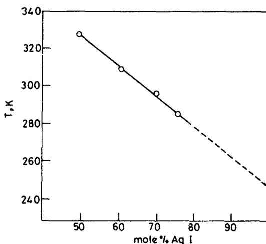
Figure 3. Variation of the glass transition temperature for the glasses in the system AgI-Ag<sub>2</sub>SeO<sub>4</sub> as a function of mol% AgI.
