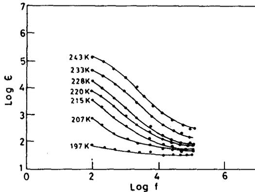
Figure 7. Variation of the real part of the dielectric constant ( $\epsilon'$ ) with frequency for the glass 50AgI-50Ag<sub>2</sub>SeO<sub>4</sub>.
