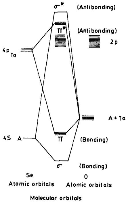
**Figure 12.** Schematic representation of the molecular orbital (MO) diagram of the  $[\text{SeO}_4]^{2-}$  ion.
