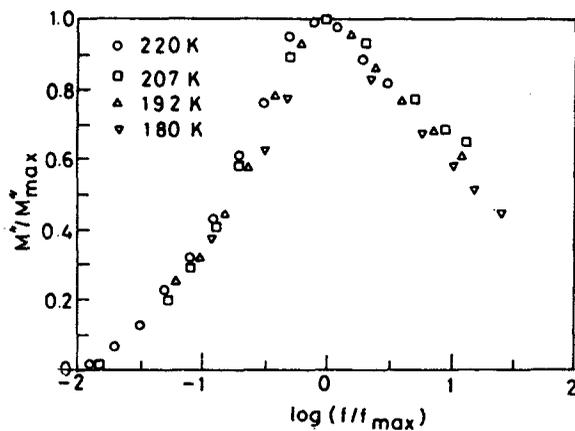
Figure 11. Plot of normalized  $M''$  against normalized frequency for the glass 50AgI-50Ag<sub>2</sub>SeO<sub>4</sub>.
