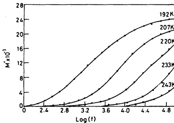
Figure 9. Variation of the real part of the electric modulus ( $M'$ ) with frequency at different temperatures for the glass 50AgI-50Ag<sub>2</sub>SeO<sub>4</sub>.
