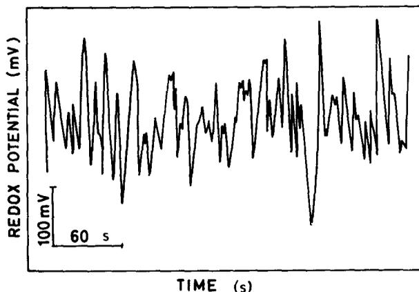
**Figure 4.** Chaotic oscillations in a continuously stirred tank reactor, thiophenol (0.012 M),  $\text{IO}_3^-$  (0.004 M),  $\text{H}_2\text{SO}_4$  (1.0 M) and  $k_0 = 0.035 \text{ min}^{-1}$  at temperature  $30^\circ\text{C}$ .
