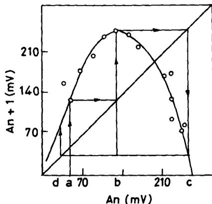
**Figure 2.** A plot of  $A(n+1)$ th oscillations amplitude against  $A$   $n$ th oscillations amplitude, thiophenol (0.012 M),  $\text{IO}_3^-$  (0.0042 M),  $\text{H}_2\text{SO}_4$  (1.0 M) at temperature  $30^\circ\text{C}$ .
