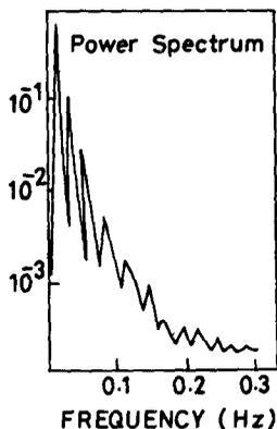
**Figure 3.** Power spectrum of the experimental data containing thiophenol (0.012 M),  $\text{IO}_3^-$  (0.0042 M) and  $\text{H}_2\text{SO}_4$  (1.0 M) at temperature  $30^\circ\text{C}$ .
