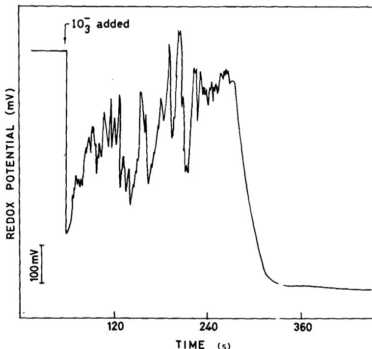
**Figure 1.** Chaotic oscillations in batch reactor, thiophenol (0.012 M),  $\text{IO}_3^-$  (0.0042 M) and  $\text{H}_2\text{SO}_4$  (1.0 M) at temperature  $30^\circ\text{C}$ .
