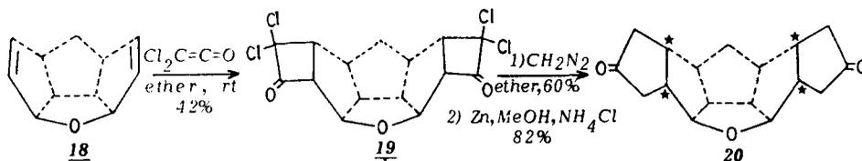
Even though *bis*-(cyclopentanone)annulation of 18 had been achieved, it could be successfully utilised for the synthesis of dodecahedrane only if the two newly appended cyclopentane rings could be projected within the cavity of the polyquinane framework. This required inversion of stereochemistry at four centres in 20 (marked with asterisks). This transformation was envisaged in a three step sequence as illustrated in scheme 8.
