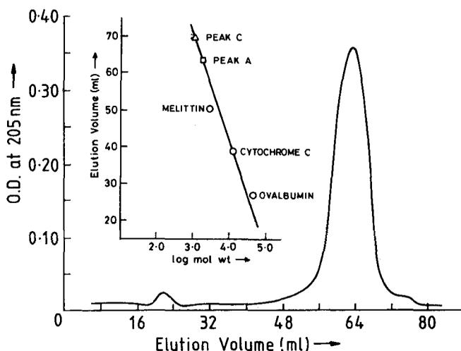
**Figure 8.** Elution profile of 60 mM cholate through the Sephadex G-50 column. Inset shows the calibration curve, for estimation of molecular weights, of the column using standard proteins. Marked on this are the peak positions of peaks A and C.
