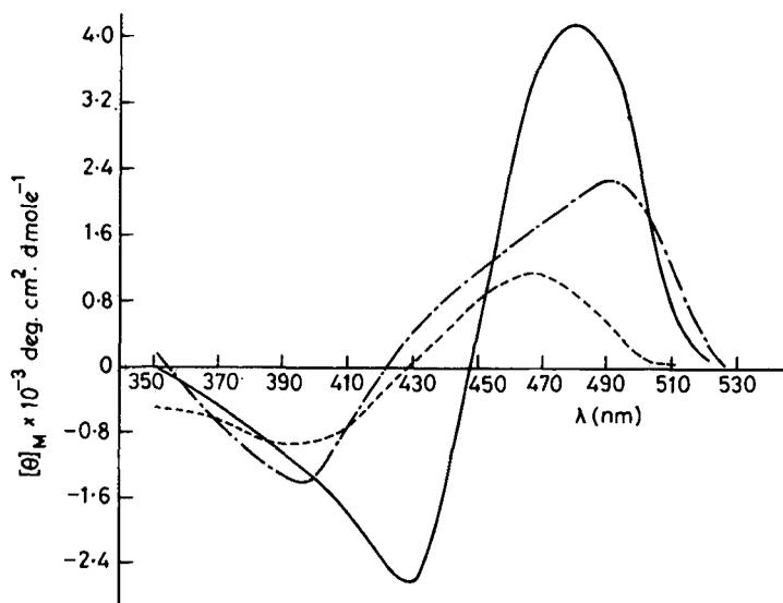
**Figure 9.** CD spectra of the column fractions. (---) peak A, pH 2.7,  $7.45 \times 10^{-6}$  M bilirubin; (—) peak B, pH 6.7,  $5.76 \times 10^{-6}$  M bilirubin; (-·-·-) peak C, pH 6.7,  $4.4 \times 10^{-6}$  M bilirubin.
