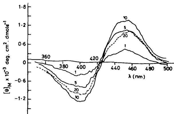
**Figure 5.** Induced CD spectrum of  $6.9 \times 10^{-6}$  M bilirubin with increasing cholate concentrations in H<sub>2</sub>O at pH 9.2 150 mM NaCl. Number over each trace is the concentration of cholate in mM.
