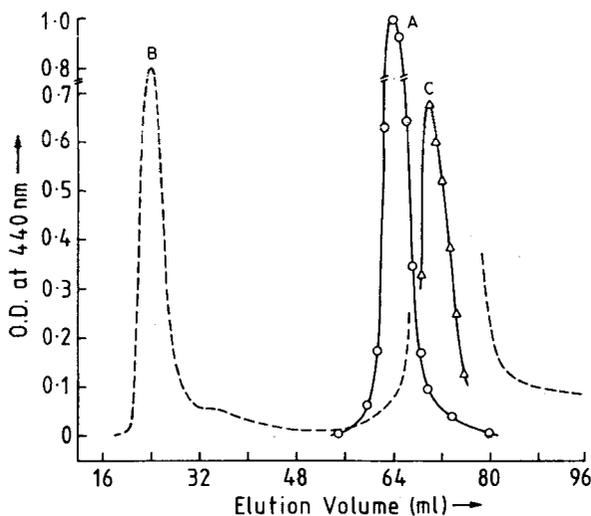
Figure 7. Elution profiles of 15 mM bilirubin in 60 mM cholate, pH 10.5 through a Sephadex G-50 column. Peak A is obtained when the eluant is H<sub>2</sub>O at pH 10.8. Peaks B and C constitute the two fractions when eluant is at pH 6.6. (Absorbances of peaks A and C are of diluted samples.)
