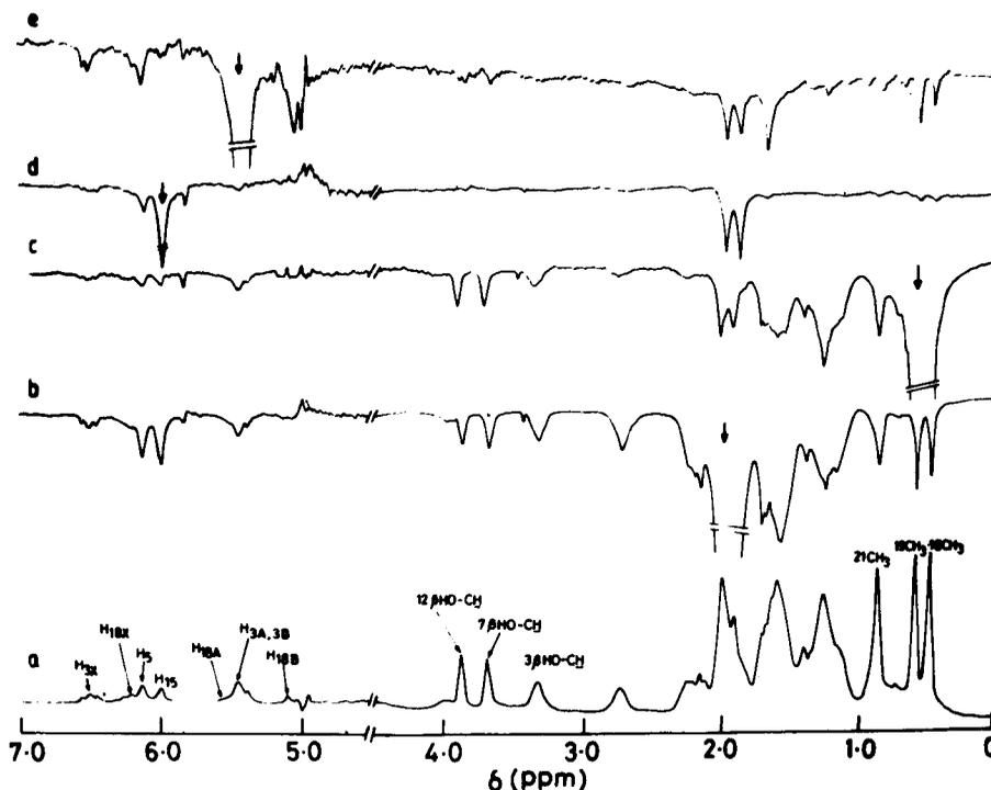
**Figure 12.** (a) 270 MHz  $^1\text{H}$  NMR spectrum of 4:1 cholate-bilirubin. (b–e) Difference NOE spectra obtained upon irradiation of the resonances indicated by an arrow. The difference NOE spectra were obtained as mentioned in the text and are magnified by a factor of 8. (Bilirubin concentration, 30 mM; cholate, 120 mM.)
