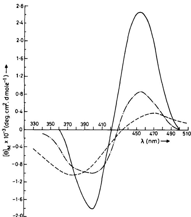
**Figure 4.** Induced CD spectra of bilirubin ( $7.6 \times 10^{-6}$  M) in the presence of 20 mM bile salts in  $\text{H}_2\text{O}$ , pH  $\sim$  10.5, 150 mM NaCl. Cholate (—), deoxycholate (---), dehydrocholate (— · —).
