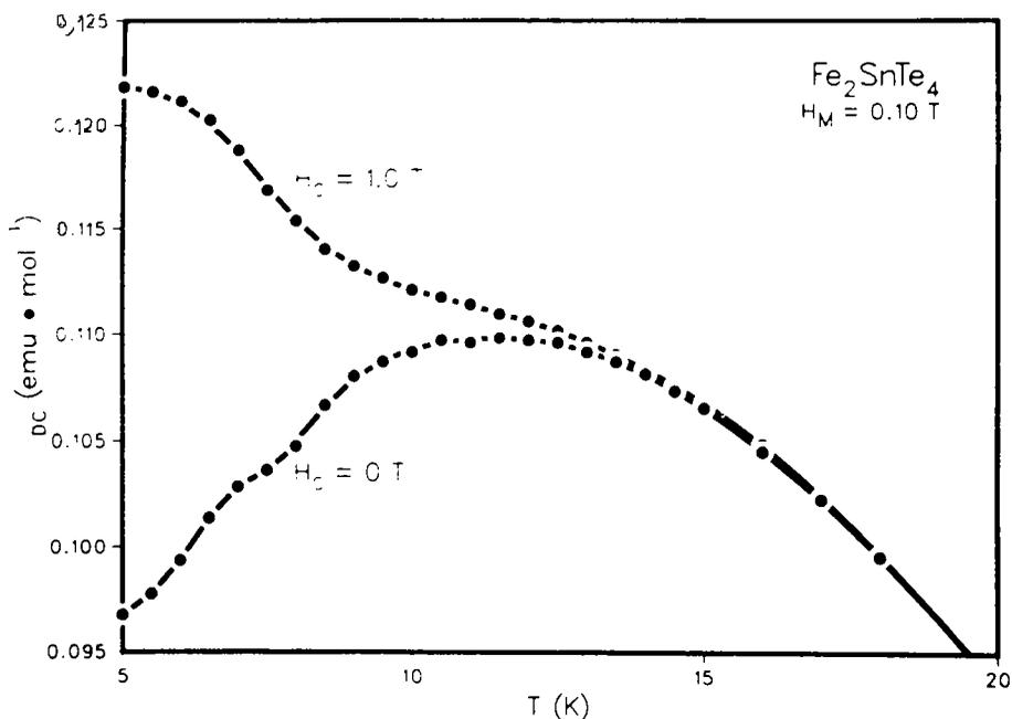
**Figure 2.** A plot of the magnetic susceptibility as a function of temperature for  $\text{Fe}_2\text{SnTe}_4$ . The two curves at low temperature illustrate the effect of zero field cooling (lower curve) and high field (1.0 T) cooling (upper curve). The two curves merge in the paramagnetic domain above the spin glass freezing temperature.
