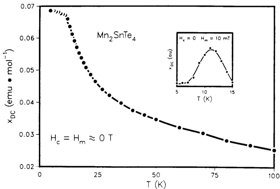
**Figure 1.** A plot of the d.c. magnetic susceptibility of  $\text{Mn}_2\text{SnTe}_4$ . The sample was frozen and measured in a field of 10 mT. The inset illustrates the magnetic response of a sample frozen at zero field and then measured at 10 mT.
