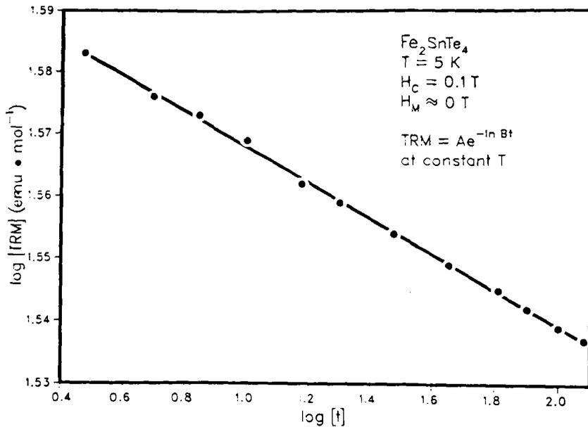
Figure 5. A log/log plot of the TRM of  $\text{Fe}_2\text{SnTe}_4$  as a function of the time.
