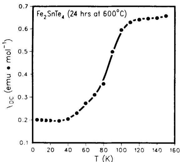
**Figure 6.** The magnetic susceptibility of a sample of  $\text{Fe}_2\text{SnTe}_4$  after it was heat treated for 24 hours at 600 K. The freshly prepared material is amorphous, while the heat treated material behaves as a mixture of  $\text{FeTe}_x$  and  $\text{SnTe}$ , where the antiferro-magnetism is attributed to  $\text{FeTe}_x$ .
