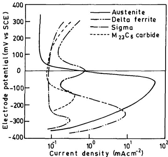
Figure 11. Anodic polarization curves in 3.6 N  $\text{H}_2\text{SO}_4$  containing 0.1 N  $\text{NH}_4\text{SCN}$ .
