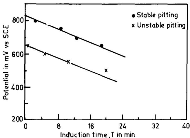
Figure 2. Plots of applied potential vs. induction time for stable and unstable pitting.
