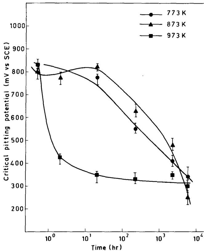
**Figure 5.** Variation in the critical pitting potential with ageing time at 773, 873 and 973 K.
