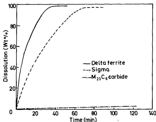
**Figure 12.** Dissolution behaviour of delta-ferrite, sigma and  $M_{23}C_6$  in 5%  $Br_2-CH_3OH$  solution.
