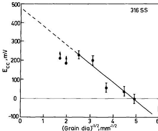
**Figure 10.** Relationship between  $E_{cc}$  and grain diameter.
