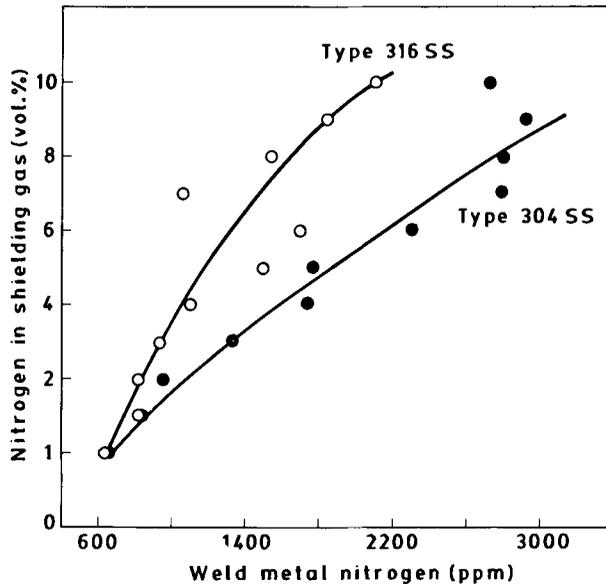
**Figure 7.** Nitrogen contents in weld metals of types 304 and 316 ss as a function of the volume percent of nitrogen gas mixed with shielding argon gas.
