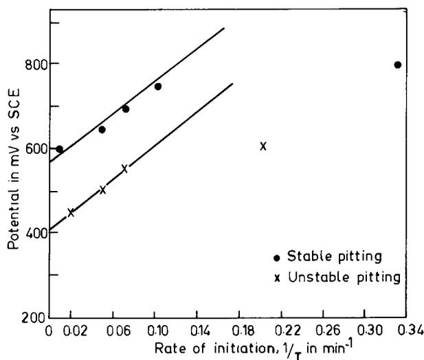
**Figure 1.** Plots of applied potential vs. rate of initiation of pits (i.e. inverse of incubation time) during stable and unstable pitting.
