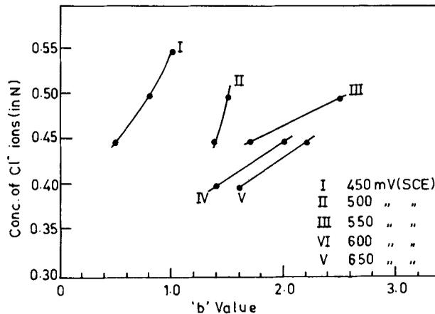
**Figure 4.** Variation of  $b$  value with respect to applied potential for different chloride ion concentrations during unstable pit growth.
