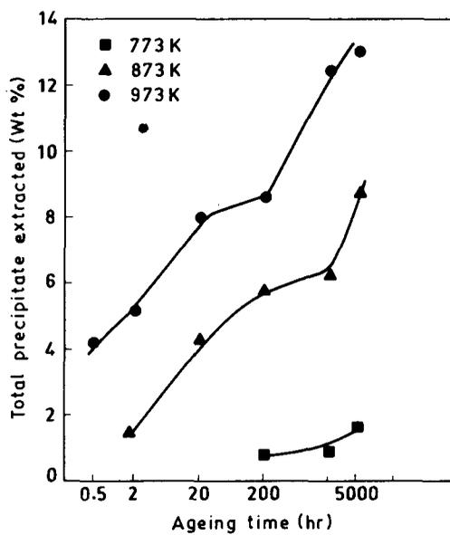
Figure 14. Total amount of precipitate extracted from the aged samples as a function of ageing time.
