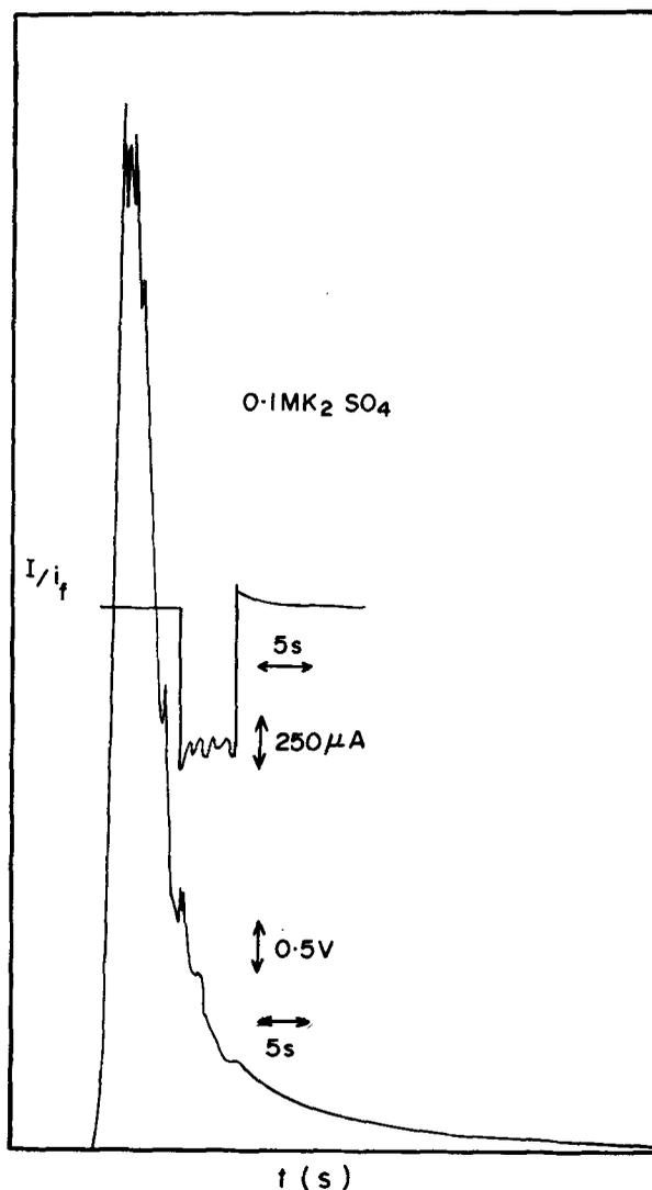
**Figure 3.** Current-time curve (at the centre) for potential step electrolysis of the *Lampito mauritii* electrode in 0.1 M  $K_2SO_4$  media. Step potential 0 to  $-1.0$  V vs SCE.  $i_f$  represents the current. Intensity-time curve during the above potential step.  $I$  = intensity.
