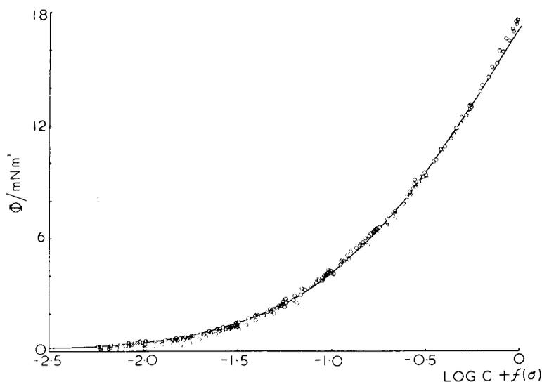
**Figure 5.** Composite surface pressure curve for xylose adsorbed on mercury in contact with 0.7953 M NaF at 25°C. The line was calculated from the Frumkin isotherm with  $a = -0.25$ ,  $\Gamma_s = 3.32 \times 10^{-10}$  mol cm<sup>-2</sup>, and  $\log \beta = 0.79$ .
