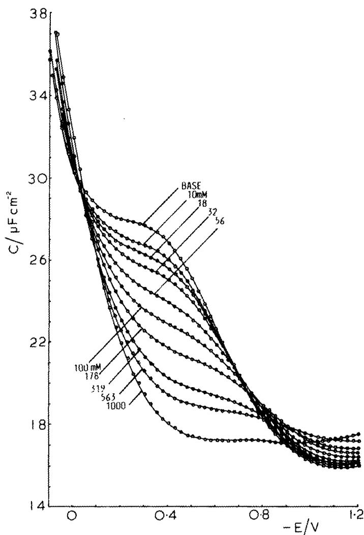
**Figure 3.** Differential capacity curves of a mercury electrode in contact with aqueous 0.7953 M NaF containing xylose. The concentration of xylose is indicated on each curve in  $\text{mmol l}^{-1}$ .
