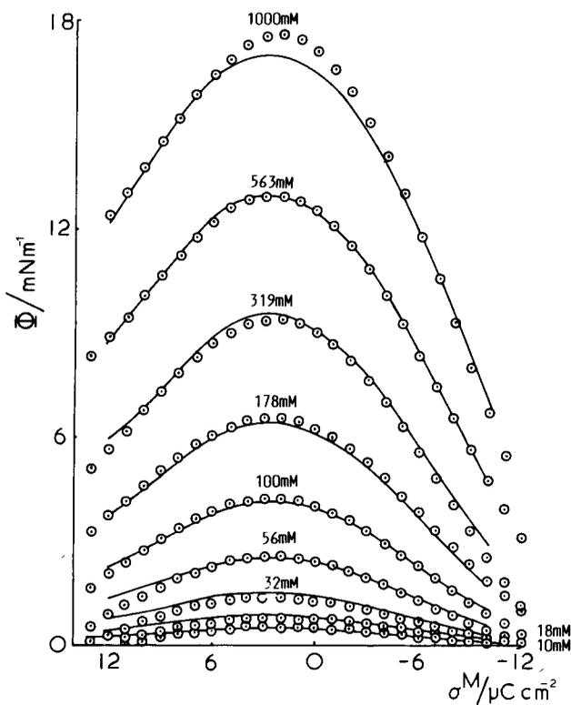
Figure 7. The surface pressure of xylose as a function of charge density on the mercury surface at 25°C. The xylose concentration in  $\text{mmol l}^{-1}$  is indicated on each curve. The lines were calculated from the Frumkin isotherm with  $a = -0.25$ ,  $\Gamma_s = 3.32 \times 10^{-10} \text{ mmol cm}^{-2}$ ,  $\log \beta = 0.79$  and experimental values of  $f(\sigma)$ .
