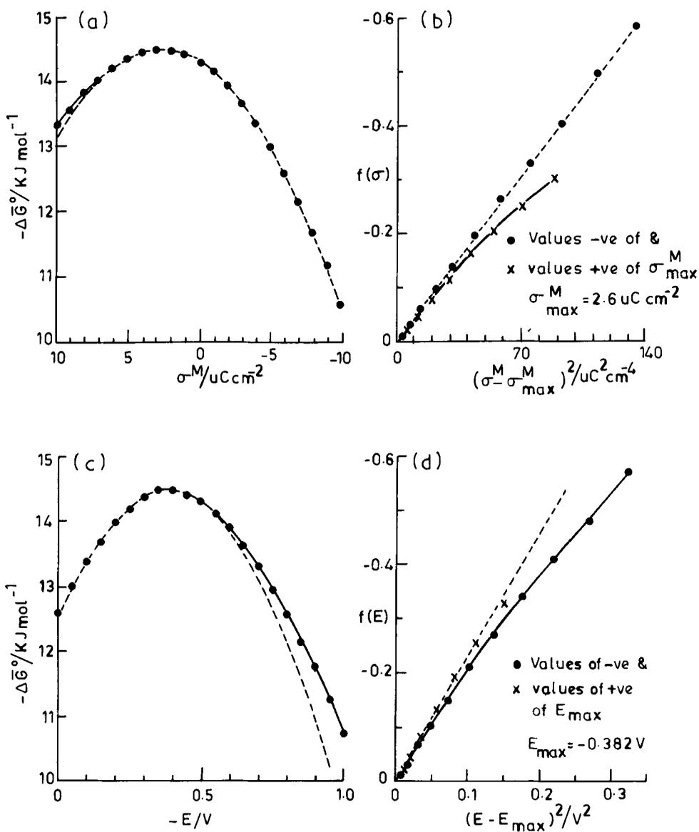
**Figure 9.** The variation of the standard Gibbs energy of adsorption of xylose with charge (a) and potential (c). The same data plotted as a function of  $(\sigma - \sigma^M)^2$  (b) and  $(E - E_{\text{max}})^2$  (d). The broken lines are calculated from (4) and (6) with  $b = 0.0043 \text{ cm}^4 \mu\text{C}^{-2}$  and  $\alpha = 2.31 \text{ V}^{-2}$  respectively.
