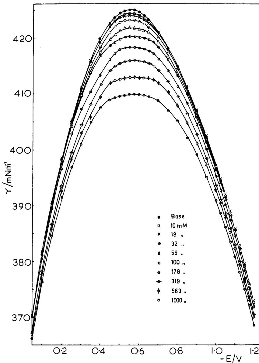
**Figure 4.** Electrocappillary curves for a mercury electrode in contact with aqueous 0.7953 M NaCl containing xylose.
