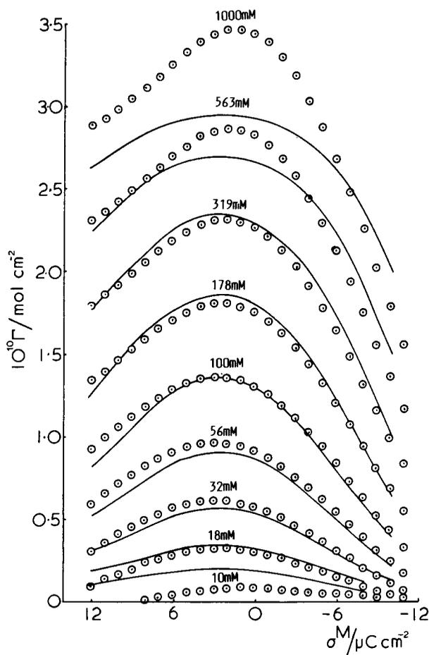
**Figure 8.** The relative surface excess of xylose as a function of charge density on the mercury surface at 25°C. The concentration of xylose in  $\text{mmol l}^{-1}$  is indicated by each curve. The lines were calculated from the Frumkin isotherm with  $a = -0.25$ ,  $\Gamma_s = 3.32 \times 10^{-10} \text{ mol cm}^{-2}$ ,  $\log \beta = 0.79$  and experimental values of  $f(\sigma)$ .
