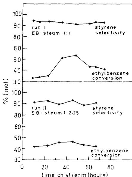
**Figure 1.** Selectivity to styrene and ethylbenzene conversion over iron oxide catalysts for run I (EB to steam ratio = 1:1) and run II (EB to steam ratio = 1:2.25) with time on stream.
