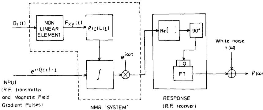
**Figure 5.** Overall system identification in terms of input (r.f. transmitter pulse and the magnetic field gradient) and response (magnetisation) as seen by the r.f. receiver. In the receiver section,  $\text{Re}[\ ]$  denotes the real, or in-phase, signal response component, and IQ denotes the imaginary, or quadrature, response component.  $n(\omega)$  denotes white noise at the output.
