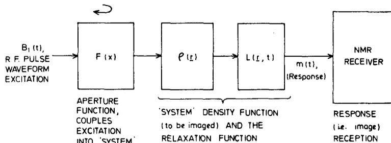
Figure 4. Excitation ( $B_1(t)$ ), Transfer ( $F(x)\rho(r)L(r, t)$ ) and Response ( $m(t)$ ) functions involved in NMR imaging. The curved arrow signifies that the 'aperture'  $F(x)$  is nonlinearly related to the r.f. excitation.
