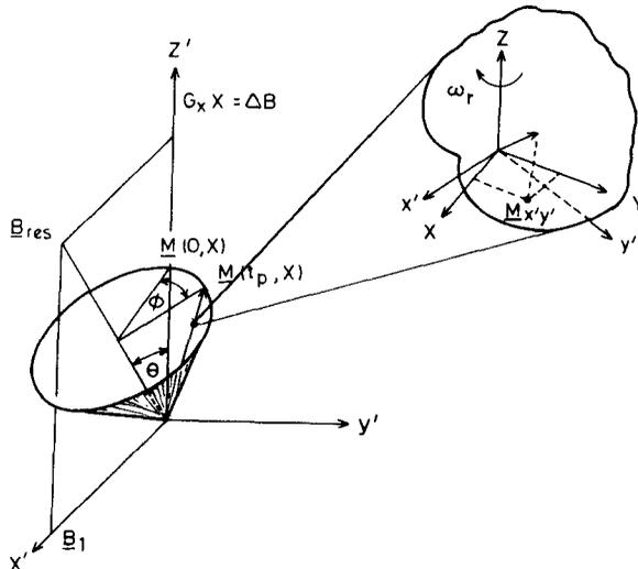
Figure 3. Precession of nuclear spin magnetisation in the rotating frame. The precession cone has its axis tilted away from  $z'$  by  $\theta$ . Exploded inset shows the projection of the instantaneous magnetisation,  $M(t_p, x)$ , onto the  $x'y'$  plane.
