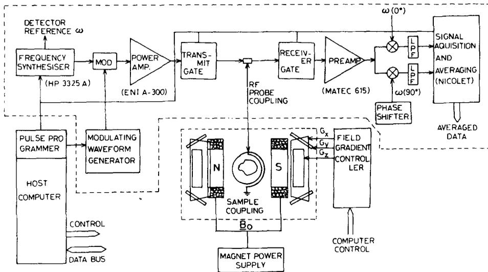
**Figure 6.** Block schematic of our NMR imaging spectrometer. The dotted section corresponds to the overall 'system' identified earlier.
