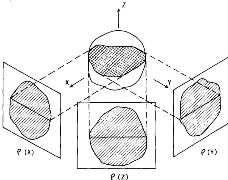
**Figure 1.** A pictorial representation of 'reconstruction', where the plane integrals are back-projected to obtain the image.
