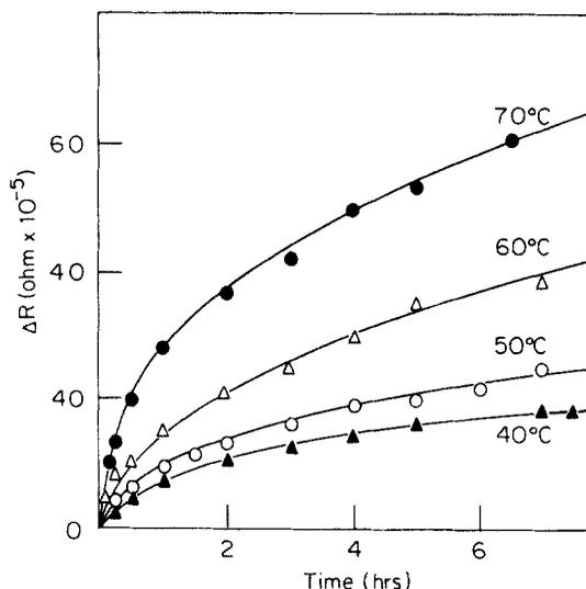
Figure 1. Kinetics of the reaction between copper (plates) and iodine (vapour) by electrical resistance measurements at different temperatures.
