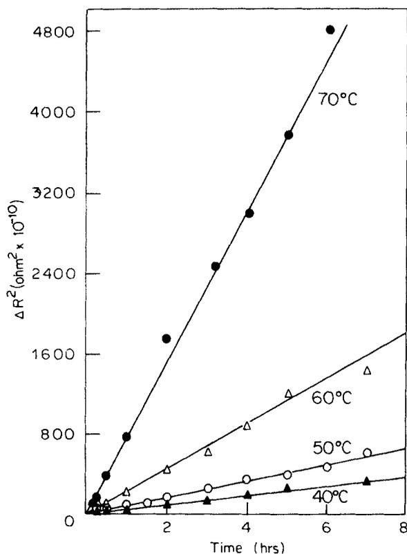
Figure 2. Plots of  $\Delta R^2$  vs  $t$  at different temperatures for the reaction between copper (plates) and iodine (vapour).
