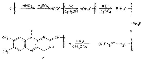
Figure 4. Reaction scheme for immobilising FAD on the graphite electrode.
