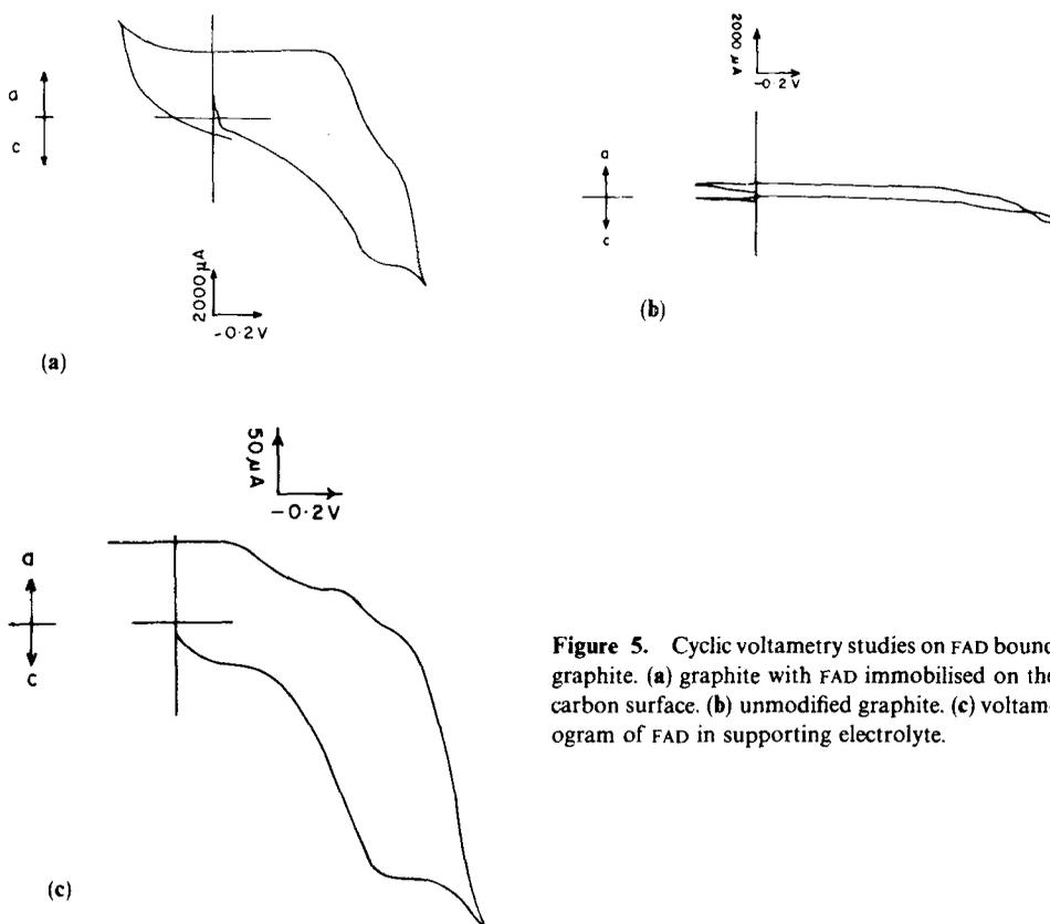
**Figure 5.** Cyclic voltammetry studies on FAD bound graphite. (a) graphite with FAD immobilised on the carbon surface. (b) unmodified graphite. (c) voltammogram of FAD in supporting electrolyte.
