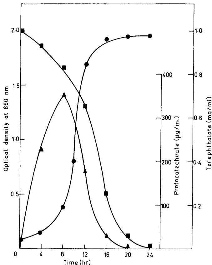
**Figure 1.** Transient accumulation of protococatechuic acid and disappearance of terephthalate from culture solution during growth of *Bacillus cirroflagellous* in 0.2% terephthalate-mineral base. Accumulation of protococatechuic acid was measured by UV analysis at 292 nm and degradation of terephthalate was measured at 241 nm. Symbols: ●—● growth; ■—■ disappearance of terephthalate; ▲—▲ transient accumulation of protococatechuic acid.
