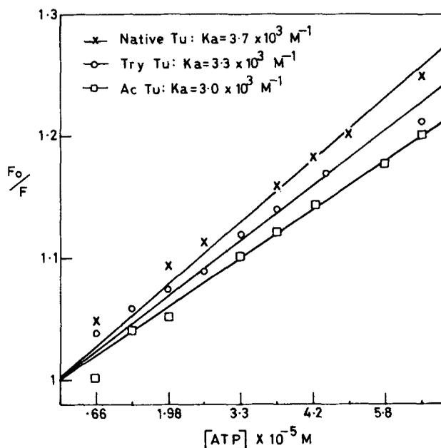
Figure 4a. Stern-Volmer plot for the association of ATP with tubulin. Tubulin taken  $10^{-6} \text{ M}$  in all three cases; - x - native tubulin; □, acetylated tubulin; ○, trypsinised tubulin.
