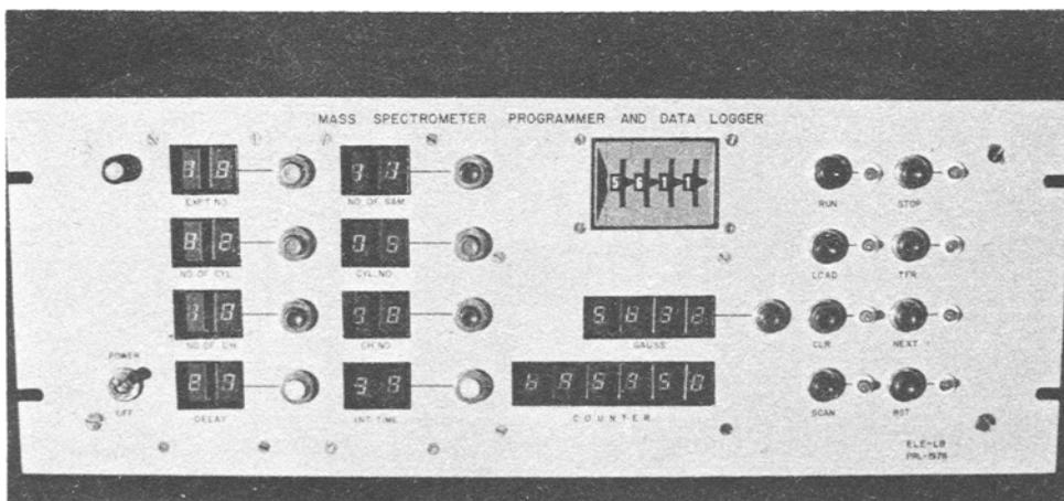
Figure 2. Front panel showing the switches for parameter entry and display.
