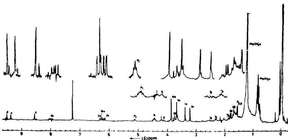
**Figure 4.** 270 MHz  $^1\text{H}$  NMR spectrum of pheophytin *a*. The numbering is the same as in figure 1. Numbers underlined indicate tentative assignments. The expanded spectrum is designated above the corresponding proton resonances.
