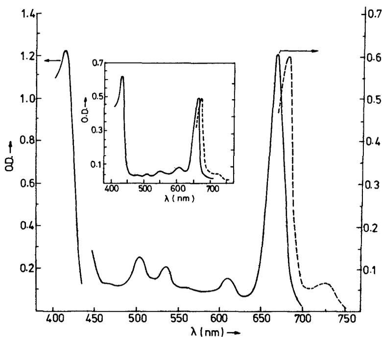
**Figure 3.** Absorption (—) and fluorescence (----) spectrum of Phe *a* in  $CH_2Cl_2$  at 25°C. Excitation at 665 nm. Inset; absorption (—) and fluorescence (----) spectrum of ZnPhe *a* in  $CH_2Cl_2$  at 25°C. Excitation at 654 nm. Fluorescence intensities are in arbitrary units.
