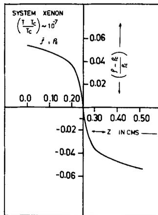
Figure 1. Density profile near the critical point.
