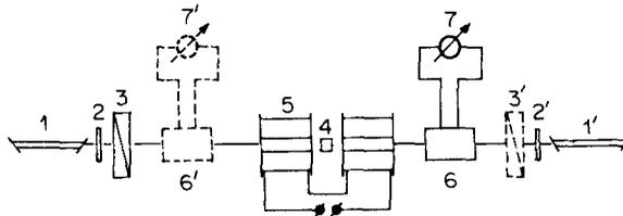
Figure 3. Block diagram of the experimental device used in studying Faraday effect and magnetogyration. 1,1'—He-Ne lasers; 2,2'— $\lambda/4$  plate in diagonal position; 3,3'—rotatable polarizer with limb; 4—sample under investigation; 5—permanent electromagnet; 6,6'—recording system; 7,7'—galvanometer.
