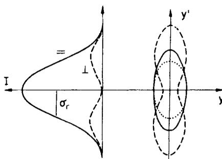
**Figure 11.** Components of the radiation distributions of one electron (left,  $\parallel$  in the orbit plane,  $\perp$  perpendicular to the plane). Synchrotron radiation source in phase-space (right, vertical distributions). The dotted line is the  $1\sigma$ -contour for the electron beam. The solid line is the contour of the parallel component, and the broken line that of the perpendicular component.
