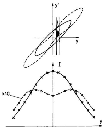
**Figure 12.** The phase-space diagram at distance  $z$  from the source; the figure is obtained from figure 11 by  $y \rightarrow y + y'z$ . The shaded rectangle shows the effective area of reflection from a small crystal, and the arrow indicates the angular scan. The lower part shows the measured average distributions of the parallel and perpendicular components across the beam.
