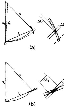
**Figure 8.** Ewald construction for diffraction from a type-I crystal (a) and a type-II crystal (b). The broken lines in (a) show the effect of variation of the incident beam direction. The inserts illustrate the active volume of the diffraction domain, when  $\Delta\epsilon$  is the divergence of the incident beam.
