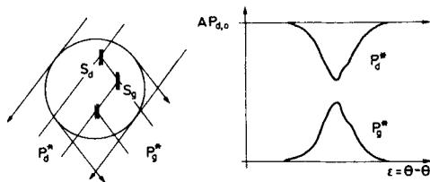
**Figure 3.** Crystal bathed in the incident beam. *P<sub>d</sub><sup>\*</sup>* is the measured power of the direct beam and *P<sub>r</sub><sup>\*</sup>* that of the reflected beam, and *AP<sub>d,o</sub>* is the transmitted beam when there is no diffraction. By conservation of energy, *P<sub>r</sub><sup>\*</sup> + P<sub>d</sub><sup>\*</sup> = AP<sub>d,o</sub>*.
