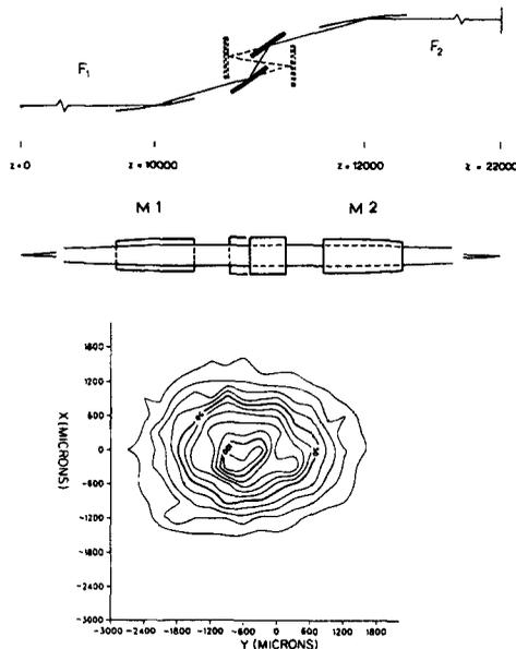
**Figure 10.** Schematic construction of an sXR beam line with 1 : 1 focussing. *M1* and *M2* are horizontally focussing grazing incidence mirrors, and the two-crystal monochromator is designed to retain the beam position. The distances *z* are in mm and typical for an x-ray beam line. The lower part shows an intensity distribution at the sample site, as obtained from a ray-tracing calculation (Hastings *et al* 1983).
