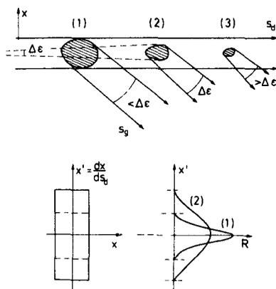
**Figure 7.** Reflection of a beam with divergence  $\Delta\epsilon$  from coherent domains of variable size. In the lower part, the width  $x$  and divergence  $x' (= \epsilon)$  of the beam are illustrated as a phase-space diagram together with the reflectivity curves of domains (1) and (2).
