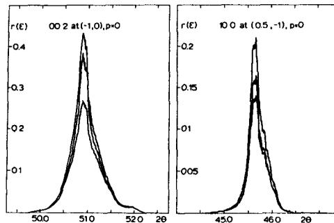
**Figure 6c.** Reflecting ratio of the measurements with polarized  $\text{CuK}\alpha$  radiation. The lowest curve is the measured profile  $r^*(\epsilon)$  when  $C = 1$ , the middle one,  $r(\epsilon)$ , is corrected for secondary extinction, and the top curve is the kinematical reflection profile calculated from the comparison with the measurement with  $C = |\cos 2\theta|$ . The scale is the same as in figure 6a.
