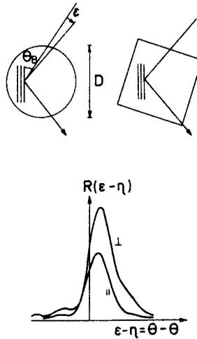
Figure 2. Regularly shaped coherent domains of size  $D$ , and typical reflectivity curves of a domain for perpendicular and parallel polarizations of the incident plane wave.
