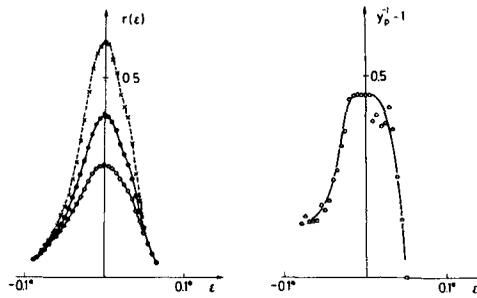
Figure 6d. Reflecting ratios for Si(111) measured with unpolarized  $\text{AgK}\beta$  (filled circles, ●) and  $\text{MoK}\alpha_1$  (open circles, ○). For details, see the legend of figure 6a.
