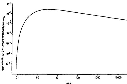
**Figure 9.** Universal spectral curve for synchrotron radiation from a bending magnet of an electron (positron) storage ring. The numbers correspond to unit of horizontal divergence (mrad), electron beam current (mA), and electron energy (GeV). The flux is integrated over the vertical divergence, and  $\lambda_c$  is the characteristic wavelength, which corresponds to the median of the power distribution.
