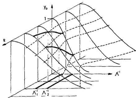
**Figure 13.** Primary extinction factor  $y_p$  as a function of the rocking angle  $\varepsilon$  of the crystal and the extinction length  $\Lambda$ . The domain size  $\delta = \delta(\varepsilon)$  is largest at  $\varepsilon = 0$ . The divergence of the beam  $\Delta\varepsilon$  makes the measurement cover a corresponding range of  $y_p$ -values (thick lines), shown for two values of  $\Lambda$ .
