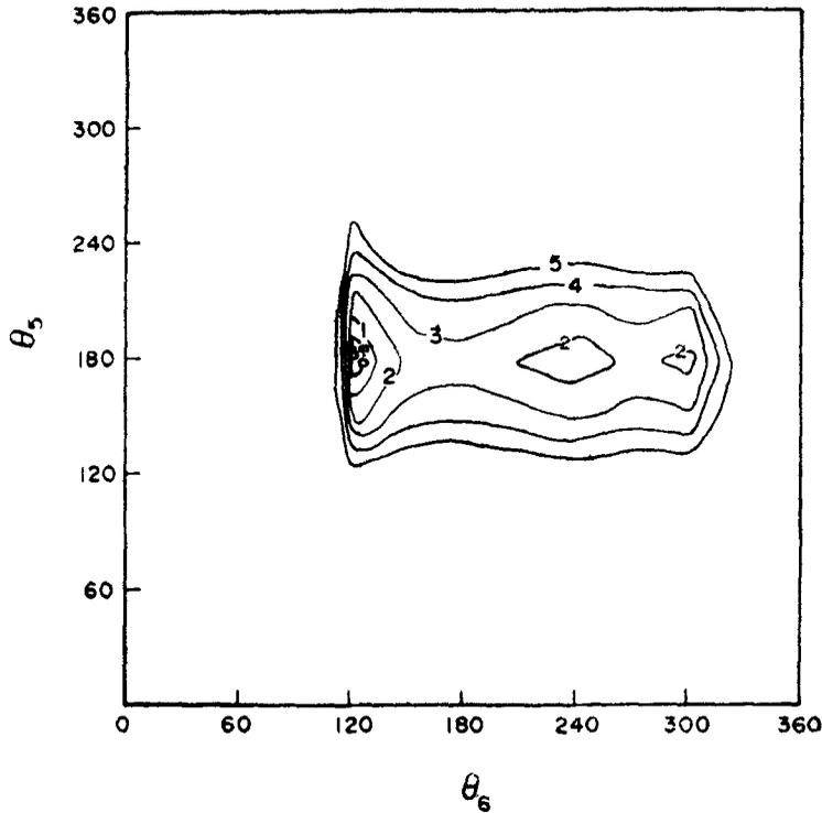
Figure 8. The  $(\theta_6 - \theta_5)$  conformational energy map for protonated Schiff base of 13-*cis* retinal constructed with  $\theta_7 = \theta_8 = \theta_9 = 300^\circ$  Isoenergy curves in kcal/mole with the global minimum taken as energy zero.
