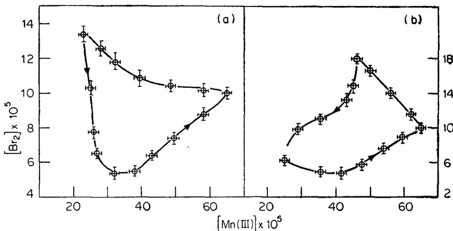
Figure 3. Experimental limit cycles: concentration conditions:  $KBrO_3$  0.05 M;  $MnSO_4$  0.005 M;  $H_2SO_4$  1.0 M; T 27°C (a) citric acid 0.05 M, (b) malic acid 0.1 M.
