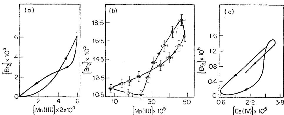
Figure 2. Limit cycles: (a) computed limit cycles from the suggested mechanism; (b) experimental limit cycle. Concentration conditions:  $KBrO_3$  0.05 M;  $MnSO_4$  0.005 M;  $H_2SO_4$  1.0 M; malonic acid 0.02 M; T 27°C; (c) limit cycle constructed from Edelson's work.
