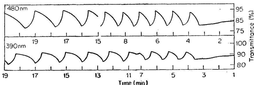
**Figure 1.** Spectrophotometric oscillations in the bromate system. Concentration conditions :  $\text{KBrO}_3$  0.05 M;  $\text{MnSO}_4$  0.005 M;  $\text{H}_2\text{SO}_4$  1.0 M; malonic acid 0.02 M; T 27° C.
