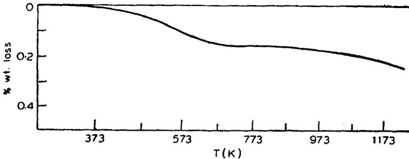
Figure 4. TGA curve of  $\text{LaNi}_{0.9}\text{Fe}_{0.1}\text{O}_3$ .
