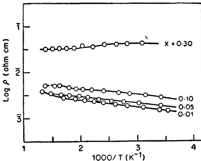
Figure 1. Plot of logarithm of electrical resistivity versus reciprocal of absolute temperature for  $\text{LaNi}_{1-x}\text{Fe}_x\text{O}_3$ .
