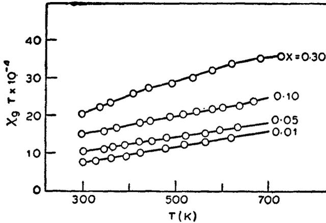
Figure 3. Variation of  $\chi T$  with temperature in  $\text{LaNi}_{1-x}\text{Fe}_x\text{O}_3$ .
