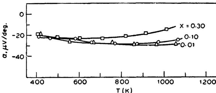
Figure 2. Variation of Seebeck coefficient with temperature in  $\text{LaNi}_{1-x}\text{Fe}_x\text{O}_3$ .
