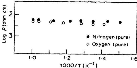
Figure 5. Plot of logarithm of electrical resistivity against reciprocal of absolute temperature for  $\text{LaNi}_{0.9}\text{Fe}_{0.1}\text{O}_3$ .
