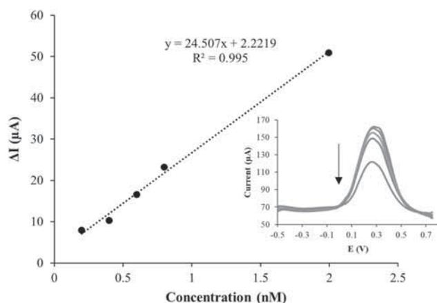
**Figure 6.** Plot of oxidation peak current vs BPA concentrations. Inset: DPV curves obtained for the proposed aptasensor recorded in 0.1 M PBS solution after incubation with different concentrations of BPA (from a to i): 0.2–2 nM.
