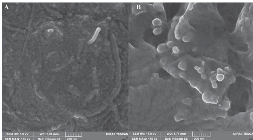
**Figure 1.** Typical FESEM images of MWCNTs-COOH,CHIT/GCE (A) and aptamer/Comp. Str./MWCNTs-COOH,CHIT/GCE (B).
