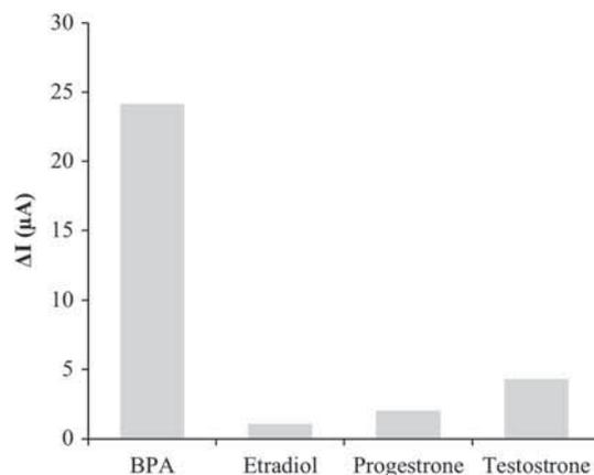
**Figure 7.** Aptasensor selectivity to BPA molecules and some interference including testosterone, estradiol and progesterone.
