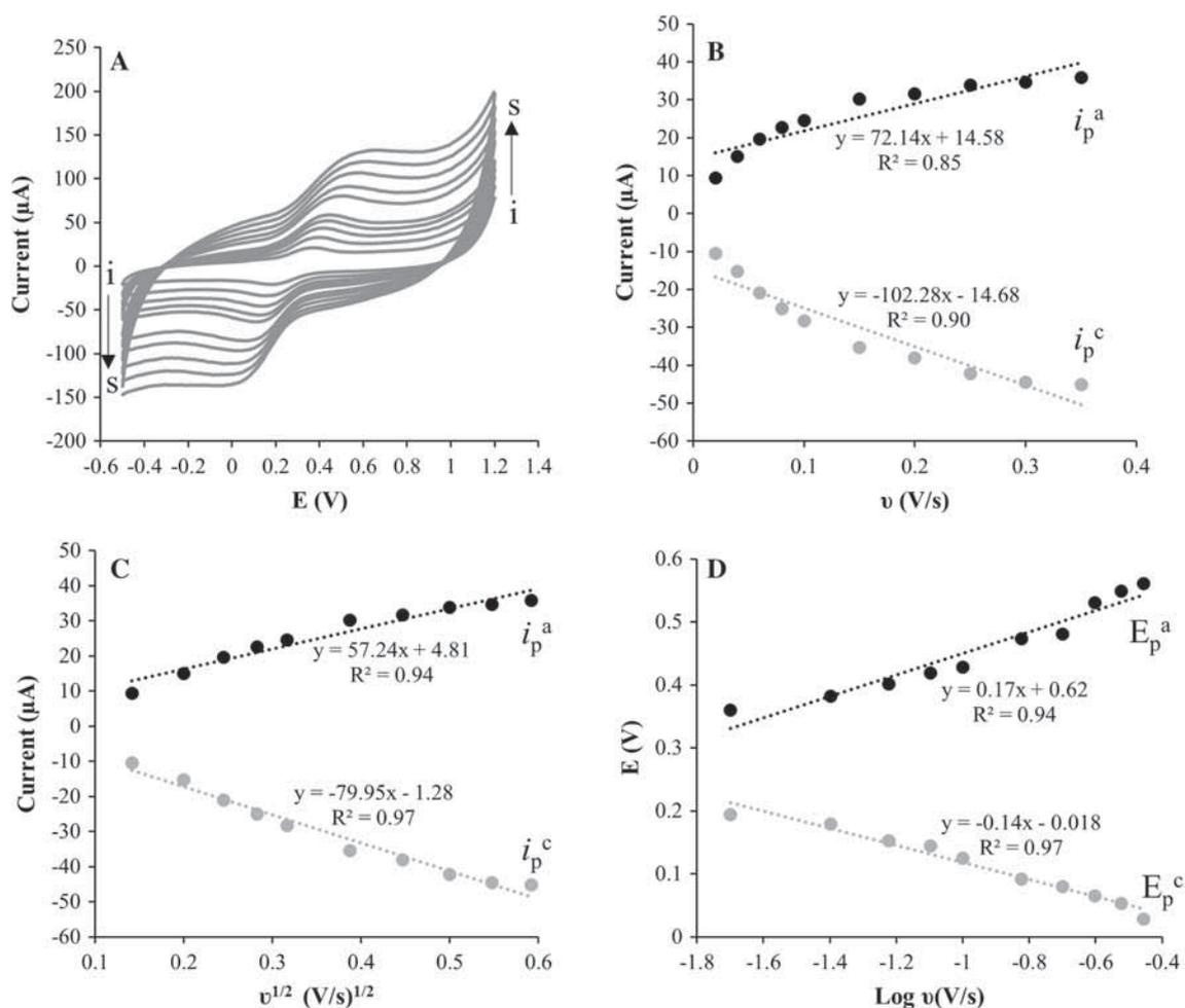
**Figure 5.** (A) Cyclic voltammograms of BPA/aptamer/Comp. Str./MWCNTs-COOH,CHIT/GCE in 0.1 M PBS pH 7.0 at different scan rates. Scan rates from (i) to (s) are 0.02, 0.04, 0.06, 0.08, 0.1, 0.15, 0.2, 0.25, 0.3 and 0.35 V/s. (B) The effect of scan rate on anodic and cathodic currents vs the scan rate. (C) The effect of scan rate on anodic and cathodic currents vs the square of the scan rate. (D) Dependence of peak potentials vs the logarithm of the scan rate.
