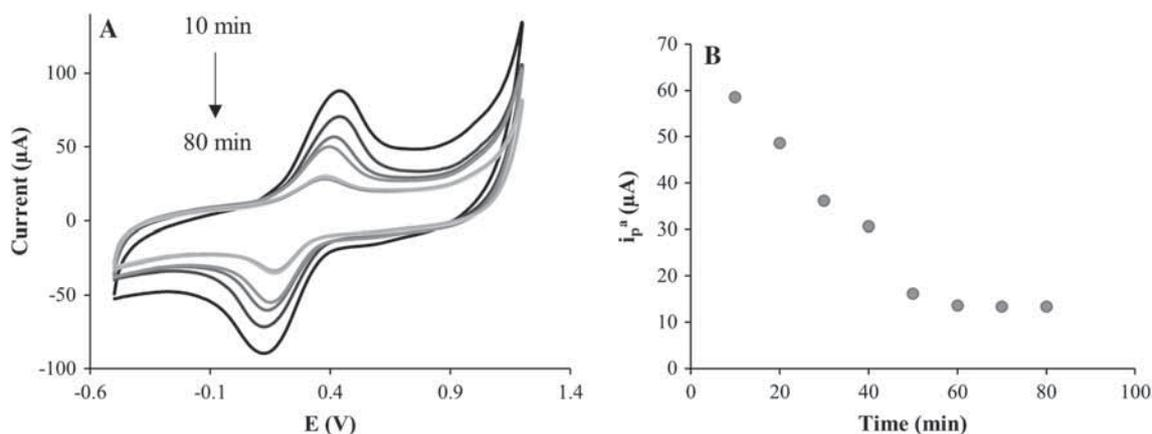
**Figure 4.** Optimization of incubation time between aptamer and BPA in 0.1 M PBS (pH 7) at a scan rate of 0.1 V/s: (A) CV curves and (B) linear plot of peak currents vs time incubation.
