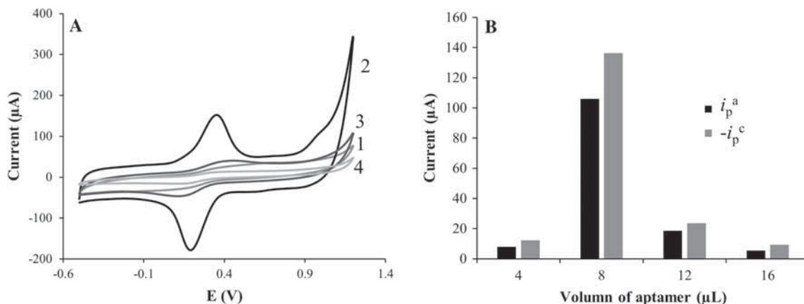
**Figure 3.** Optimization of aptamer volume in 0.1 M PBS (pH 7) at a scan rate of 0.1 V/s: (A) CV curves: 4  $\mu\text{L}$  (curve 1), 8  $\mu\text{L}$  (curve 2), 12  $\mu\text{L}$  (curve 3) and 16  $\mu\text{L}$  (curve 4). (B) Bar chart of peak currents vs aptamer volumes.
