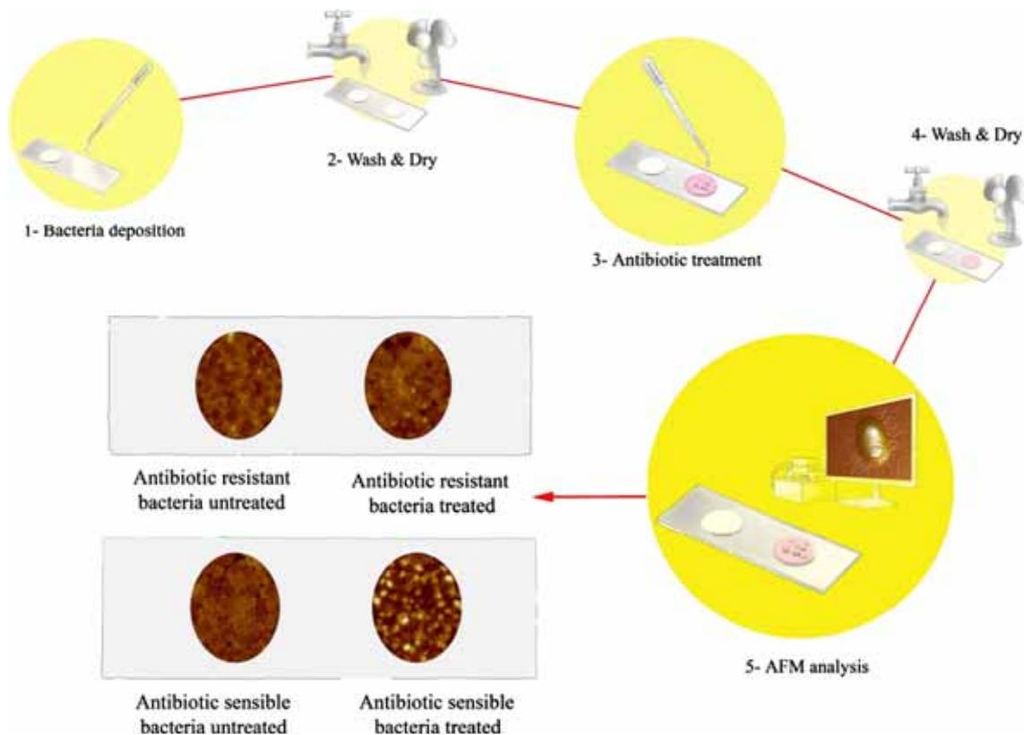
**Figure 2.** Specimens preparation scheme.
