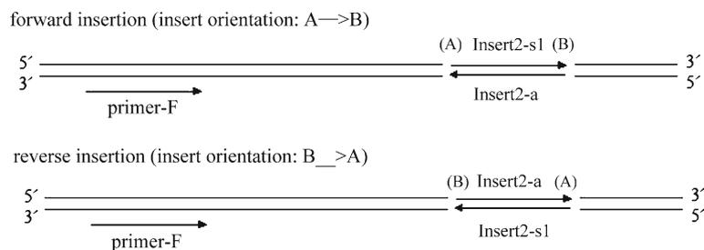
**Figure 6.** Schematic of identifying forward or reverse insertions by PCR. Insert is composed of oligonucleotides insert2-s1 and insert2-a. The ends of insert duplex are labeled with 'A' and 'B'. The orientations of insertion are demonstrated as 'A→B' for forward insertion and 'B→A' for reverse insertion.
