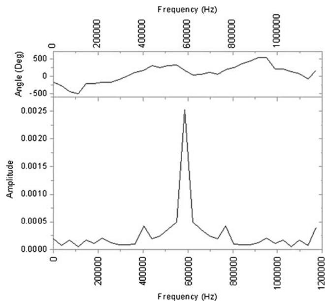
**Figure 4.** Fourier power transform of the emission data. The peak frequency is at 0.586 MHz, and upper and lower side band frequencies are at 0.769 MHz and 0.403 MHz, respectively.
