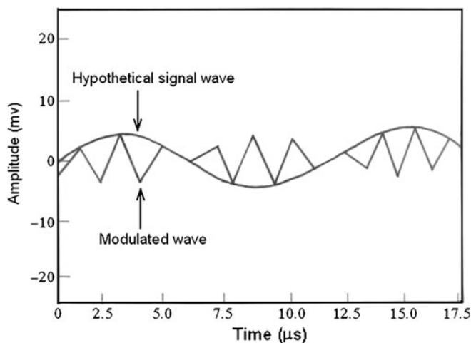
**Figure 2.** Smoothened waveform along with a hypothetical signal. Both amplitude and duration appear to be modulated according to the ‘command’ signal, exhibiting pulse amplitude modulation (PAM) and pulse width modulation (PWM).
