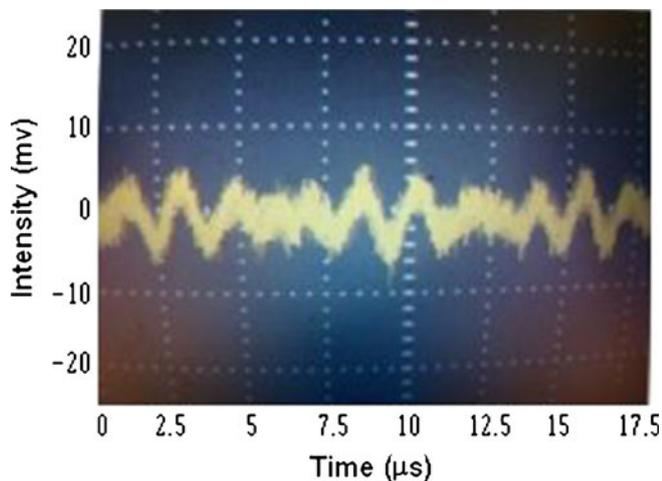
**Figure 1.** Continuous train of microsecond-duration triangular pulses recorded from an ethyl acetate-affected firefly. A set of three (and a half) pulses is a mirror image of the preceding set of three (and a half) pulses – the resultant of an oscillating chemical reaction.
