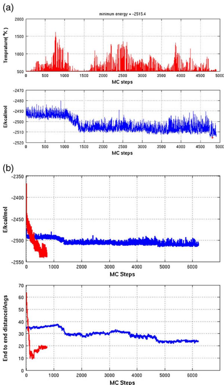
**Figure 4.** (a) Variation of temperature and energy in a representative TBP trajectory. (b) Variation of energy and end-to-end distance for two representative TBP trajectories.
