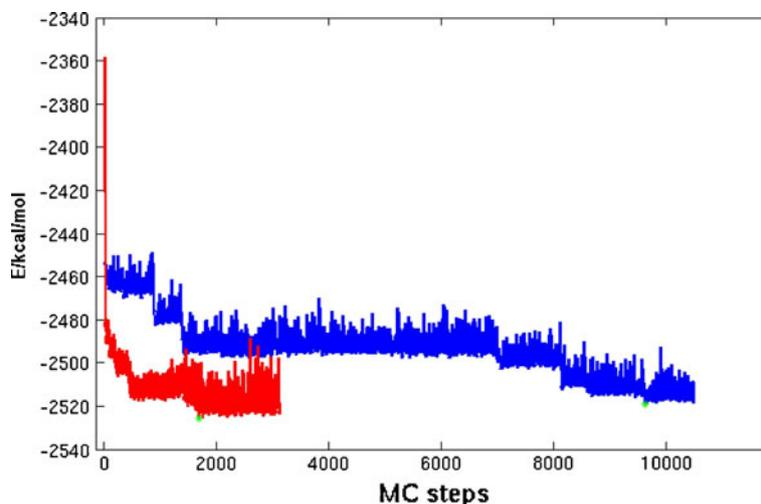
**Figure 3.** A comparison between the trajectories obtained from two different biasing terms. The blue trajectory is with only energy as the biasing term and the red trajectory is with both energy and end-to-end distance as the biasing terms.
