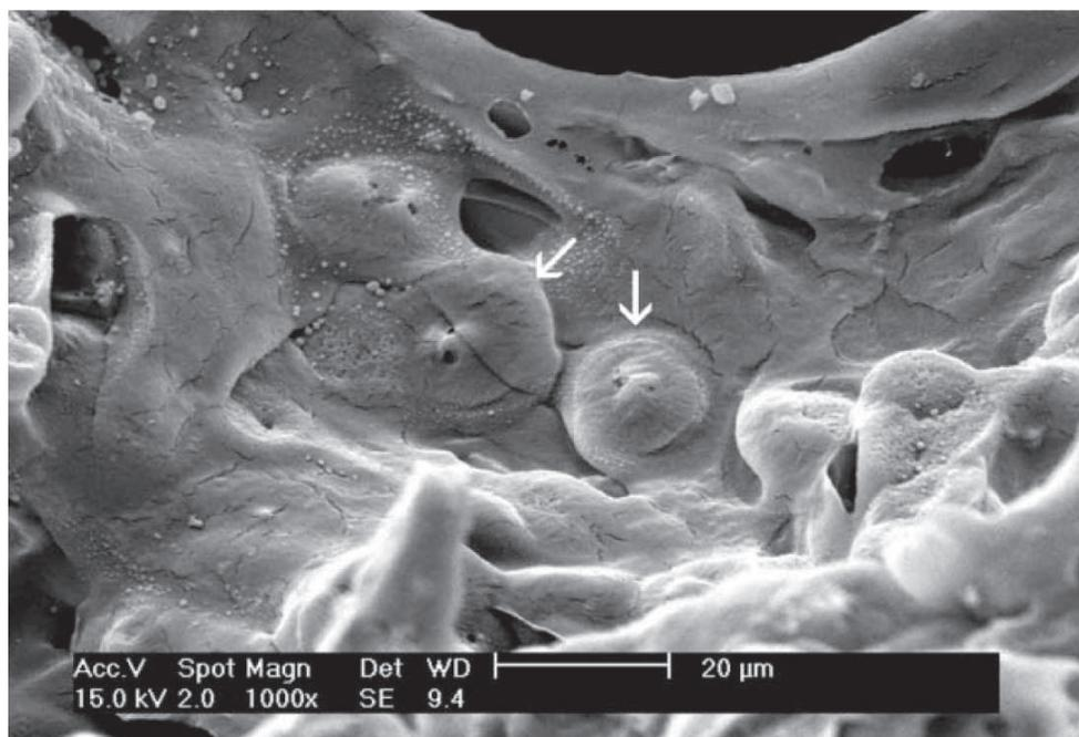
**Figure 4.** SEM micrograph of PLLA scaffold observed 2 days after cell plating. Arrows indicate the cells.
