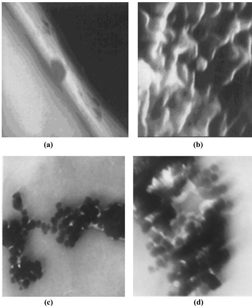
**Figure 1.** Scanning and transmission electron micrographs (TEM) of nafion and riboflavin. Scanning electron micrograph images of the nafion–riboflavin membrane: (a) cross-section, (b) top view. TEM images (c, d) of nafion–riboflavin nanoparticles. (For details, refer to the text.)
