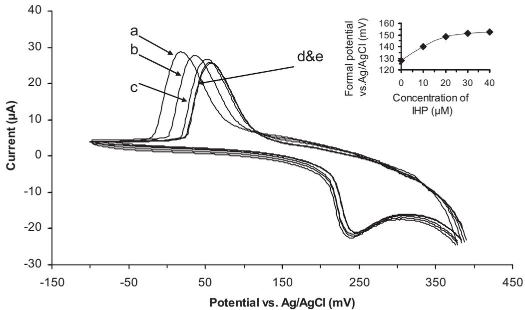
**Figure 3.** Cyclic voltammograms of haemoglobin in the presence of (a) 0, (b) 10, (c) 20, (d) 30 and (e) 40  $\mu\text{M}$  IHP. Inset shows the plot of [IHP] vs.  $E^{\circ}$ .
