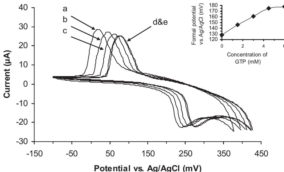
**Figure 4.** Cyclic voltammograms of haemoglobin in the presence of (a) 0, (b) 1.5, (c) 3.0, (d) 4.5 and (e) 6.0 mM GTP. Inset shows the plot of [GTP] vs.  $E^{\circ}$ .
