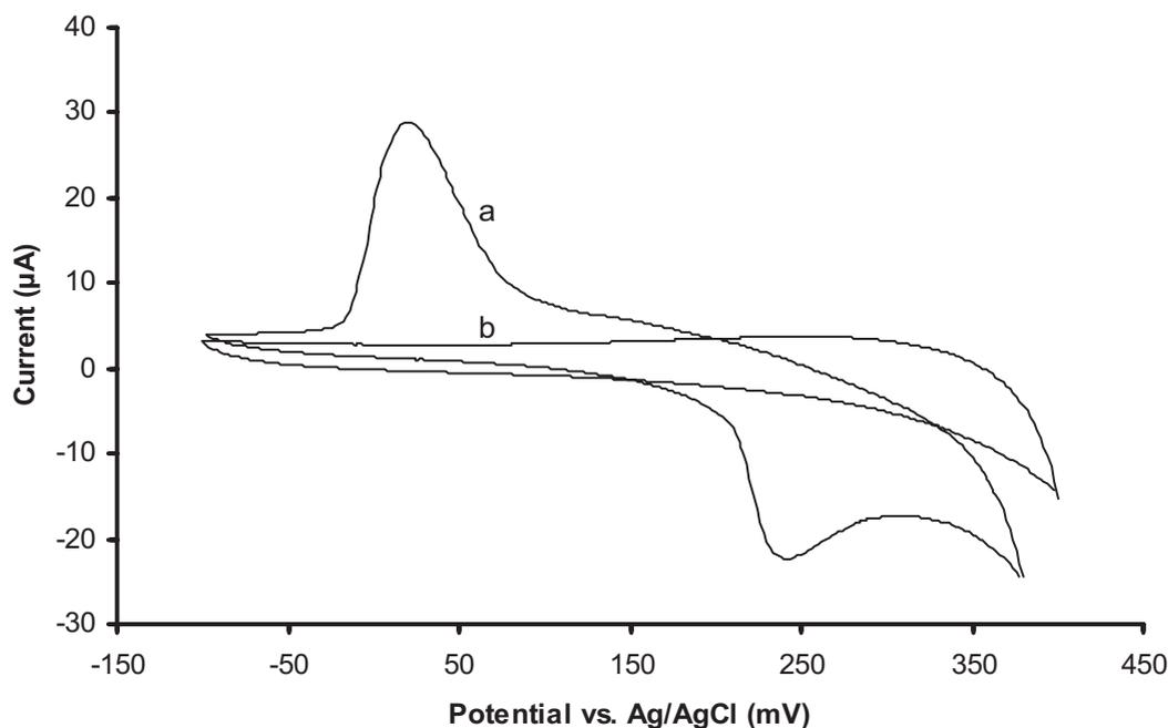
**Figure 1.** A typical cyclic voltammogram of the iodide-modified Ag electrode in  $\text{KNO}_3$  in the presence (a) and absence (b) of haemoglobin.
