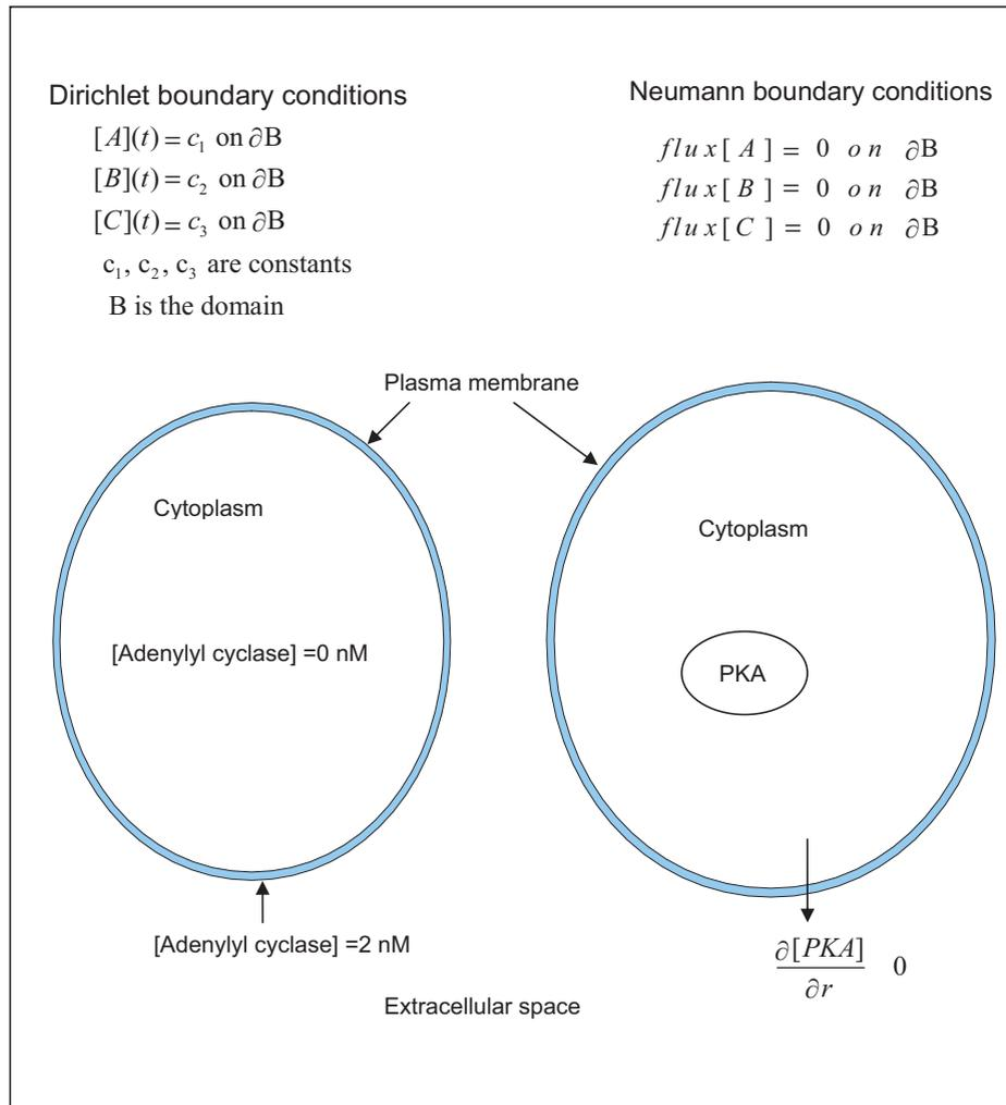
**Figure 7.** Boundary condition for PDEs. The Dirichlet boundary condition states that the value of a component is a constant on the domain boundary while the Neumann condition states that the flux of a component across the boundary is zero. Using the Dirichlet conditions we can define the concentration of adenylyl cyclase to be zero in the cytoplasm but a constant value in the membrane. Using Neumann condition, we can define the flux of PKA across the cell membrane is zero.
