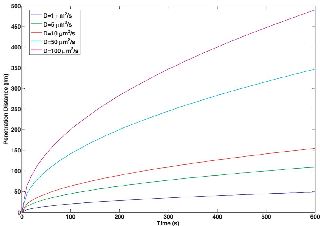
**Figure 6.** Mean displacement for different values of diffusion constants. The mean displacement is calculated for different values of diffusion coefficients over time. Even in the case of low diffusion constants, over 10 min, the mean displacement is around 50  $\mu\text{m}$ , indicating that most biochemical reactions are not diffusion-limited.
