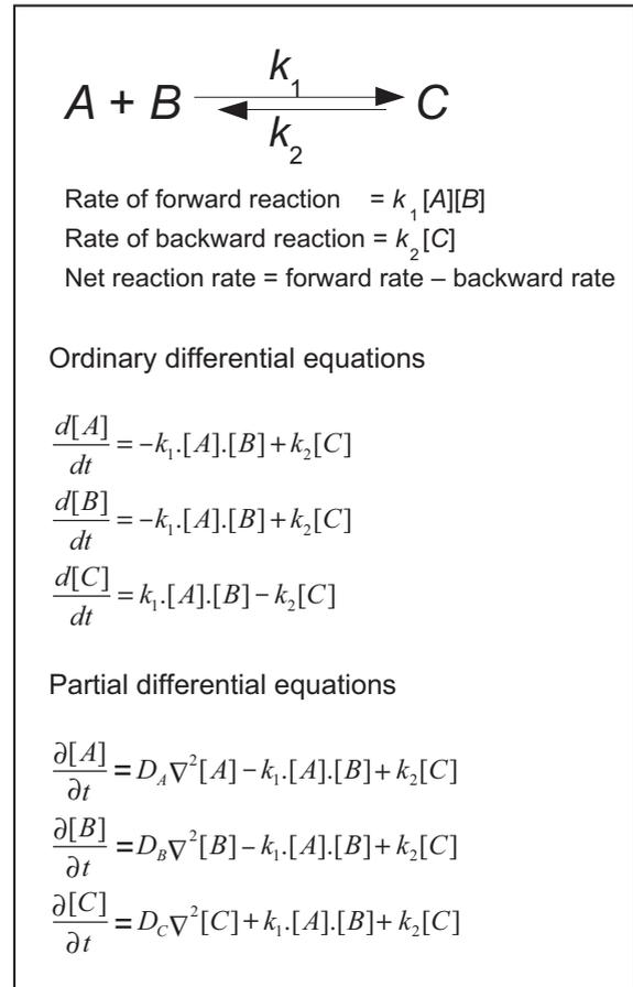
**Figure 4.** Chemical kinetics and differential equations. For a simple bimolecular reversible reaction, the reaction and the rates of forward reaction are formulated based on mass-action kinetics. Then the ordinary differential equations are formulated and subsequently the partial differential equations where  $D$  is the diffusion coefficient for a particular species.
