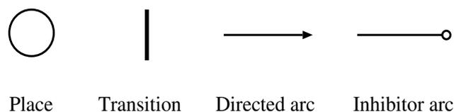
**Figure 1.** Basic elements of Petri net.
