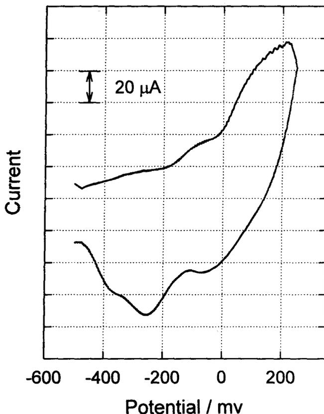
**Figure 3.** CV of enzyme electrode with adsorbed quinone in the presence of substrate (glucose) in a deoxygenated sample. The peaks due to quinone are clearly seen. Scan rate: 1 mv/s. Other conditions are similar to figure 2.
