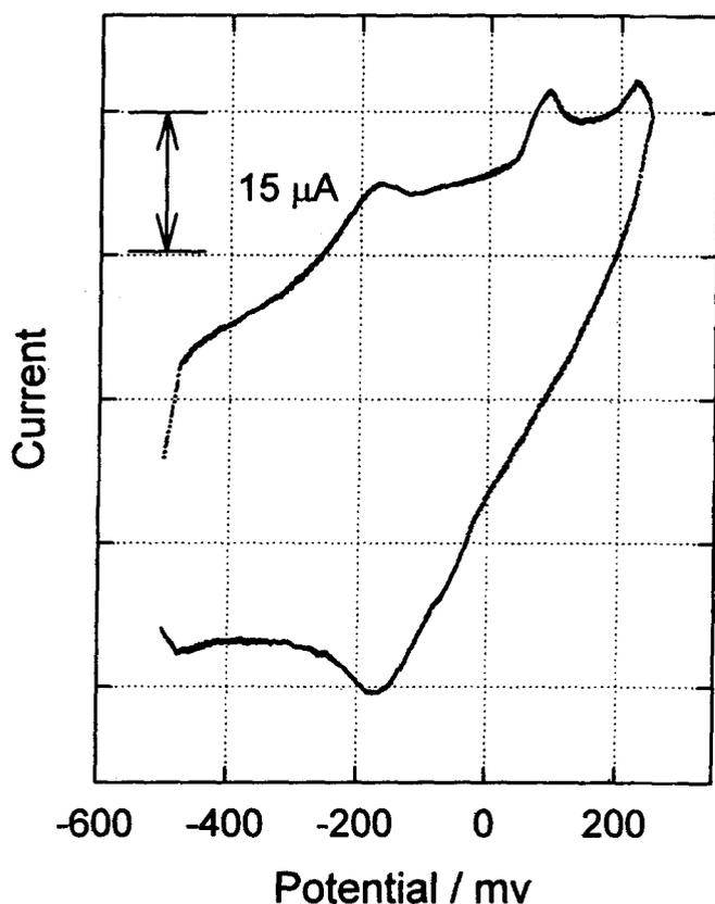
**Figure 2.** CV of enzyme electrode with two adsorbed mediators: riboflavin and quinone. Here three clear peaks are observed, one reversible peak corresponding to quinone reduction and two irreversible peaks corresponding to FAD reduction (as in figure 1). Riboflavin peaks are out of range of the potential range used. Scan rate: 2 mv/s.
