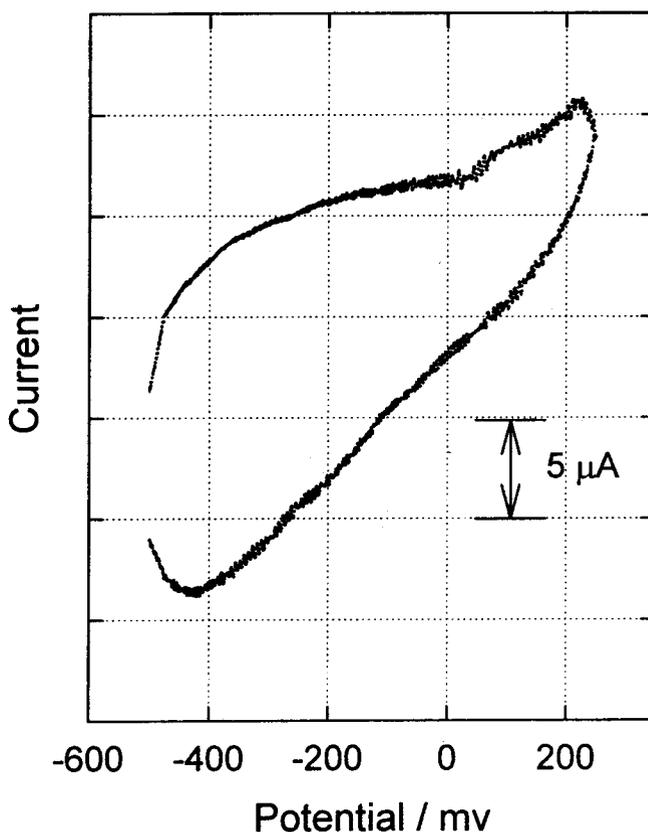
**Figure 1.** CV of enzyme electrode with no adsorbed mediator species. The potential scan was taken in the presence of glucose (1 mM). Two small irreversible peaks can be observed that correspond to the reduction of the enzyme bound FAD cofactor. Scan rate: 0.5 mV/s; electrode surface area:  $\sim 2.2$  cm<sup>2</sup>.
