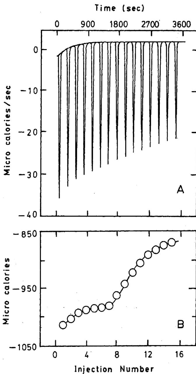
**Figure 9.** Microcalorimetric data of  $7.26 \times 10^{-6}$  M protein being titrated versus  $2.41 \times 10^{-4}$  M CGA. (A) Raw data of the energy changes in the titration cell. (B) Analysed and curve fitted data of the titration up to a titration of 15 injections over a period of 3600 s.
