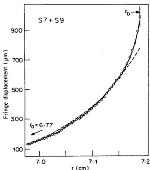
**Figure 1d.** Fringe displacement ( $\mu\text{m}$ ) *versus* radial position. Sedimentation equilibrium experiment conditions 1:1 ratio by mass (0.24 mg/ml of each) of S7: S9 at 24,000 rpm at  $3^\circ\text{C}$ . The dashed line is the best fit for two species and the solid line is the best fit for the model proposed (see text).
