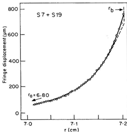
**Figure 1c.** Fringe displacement ( $\mu\text{m}$ ) versus radial position. Sedimentation equilibrium experiment conditions 1:1.4 ratio (0.25:0.35 mg/ml of each) of S7:S19 at 33,450 rpm at  $3^\circ\text{C}$ . The dashed line is the best fit for two species and the solid line is the best fit for 3 species.
