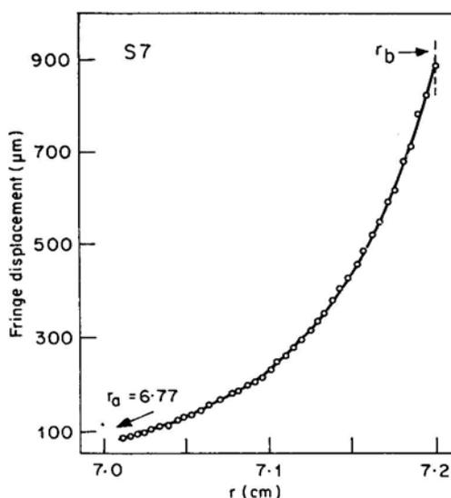
**Figure 1a.** Fringe displacement ( $\mu\text{m}$ ) versus radial position. Sedimentation equilibrium experiment conditions S7,  $0.17\text{mg/ml}$  and  $31,410\text{ rpm}$ ; solid line is best fit for a single species.
