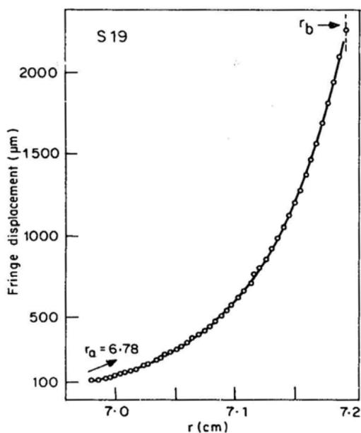
**Figure 1b.** Fringe displacement ( $\mu\text{m}$ ) *versus* radial position. Sedimentation equilibrium experiment conditions S19, 0.37 mg/ml, 36,000 rpm; solid line is the best fit for a single species.
