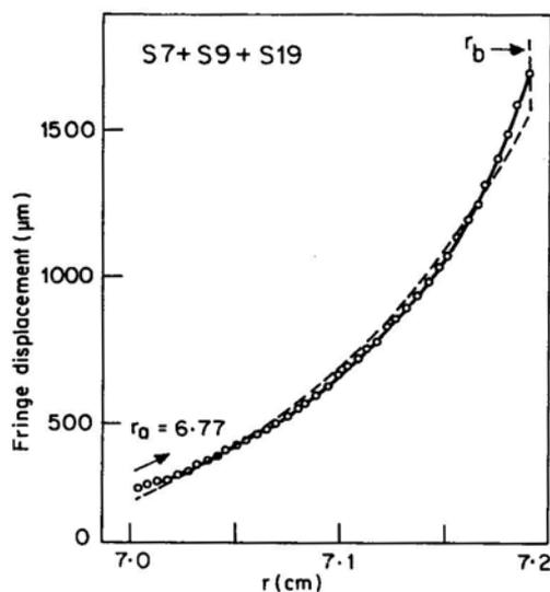
**Figure 1f.** Fringe displacement ( $\mu\text{m}$ ) *versus* radial positions. Sedimentation equilibrium experiment conditions 1:1:1 ratio by mass (0.46 mg/ml of each) S7: S9: S19 at 26,000 rpm at  $3^\circ\text{C}$ . The dashed line is the best fit for 3 species and the solid line is the best fit for the model proposed (see text).
