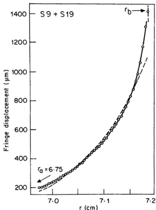
**Figure 1e.** Fringe displacement ( $\mu\text{m}$ ) *versus* radial position. Sedimentation equilibrium experiment conditions 1:1 by mass (0.30 mg/ml of each) of S9:S19 at 27,690 rpm at  $3^\circ\text{C}$ . The dashed line is the best fit for the two species and the solid line is the best fit for the model proposed (see text).
