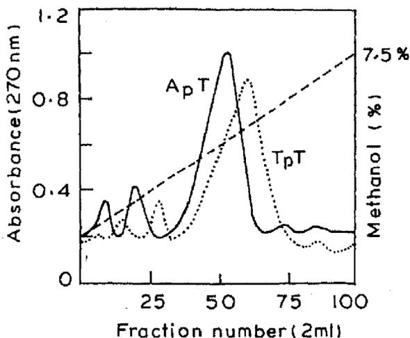
Figure 1. Column chromatography of fully protected dinucleotides.
