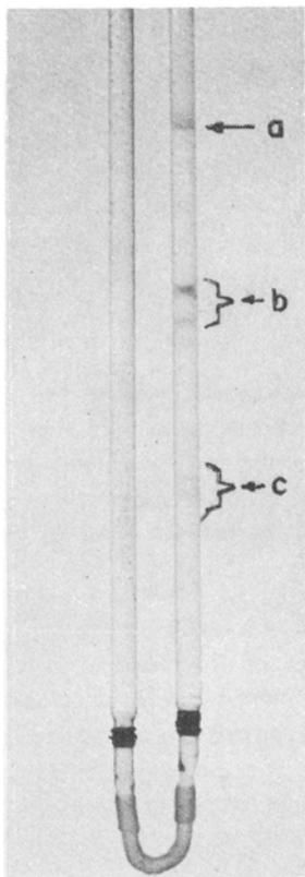
**Figure 3** Isoelectric focusing pattern of (a) cytochrome c, (b) myoglobin (two bands) and (c) ferritin (two bands).
