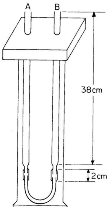
**Figure 1.** Schematic diagram of the modified electrofocusing set-up.
