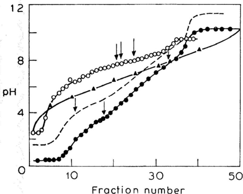
**Figure 2.** Determination of isoelectric point of (---) intracellular glucose (xylose) isomerase from *Chainia*, (○) Bandicoot haemoglobin (▲) subtilisin inhibitor from horse gram and (●) extracellular xylose isomerase from *Chainia*. Arrows indicate positions of focused proteins in pH gradient.
