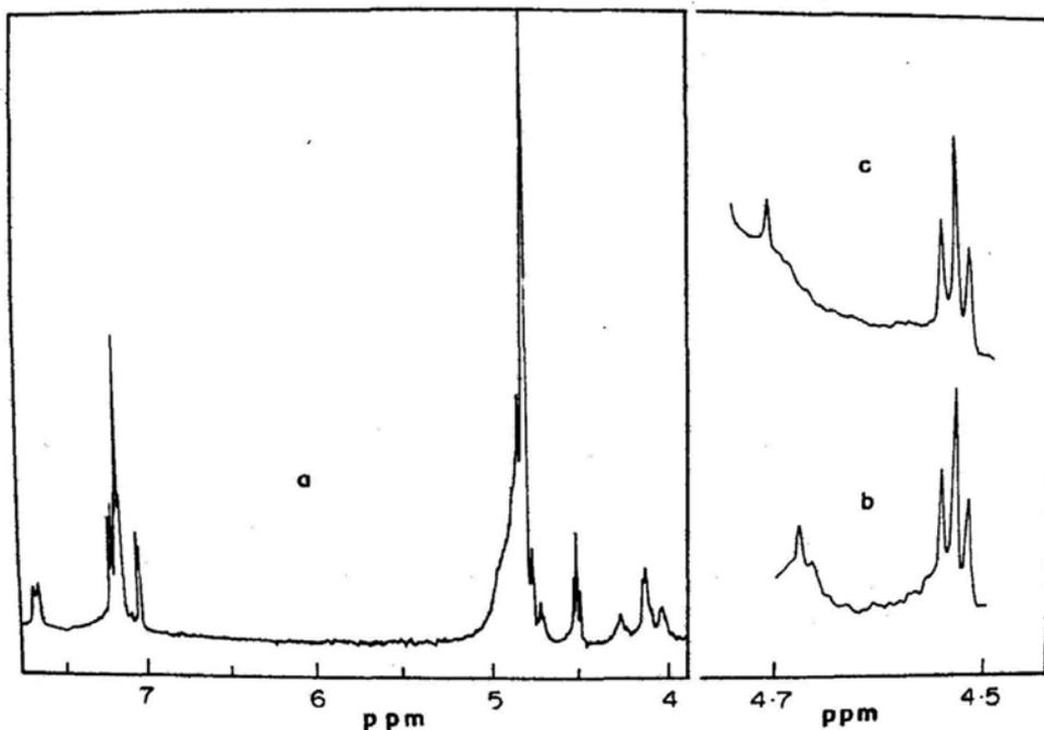
**Figure 3.** 1D-NMR spectrum of CLPA (1 mM) in CD<sub>3</sub>OD in the presence of TbCl<sub>3</sub> (0.3 mM). (a), Downfield region of the system; (b), the  $\alpha$ -CH region; (c), is the  $\alpha$ -CH region with double irradiation at 7.18 ppm.
