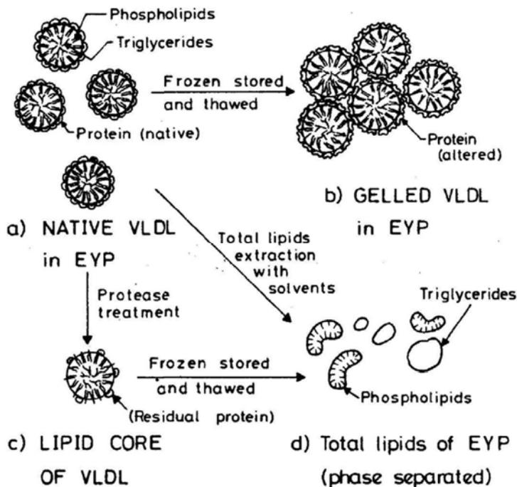
**Figure 5.** Schematic representation of lipid and protein association. (a), Native VLDL particles; (b), freeze damaged and gelled VLDL particles; (c), 'lipid core' particles obtained by protease treatment; (d), phase separated, total lipids.
