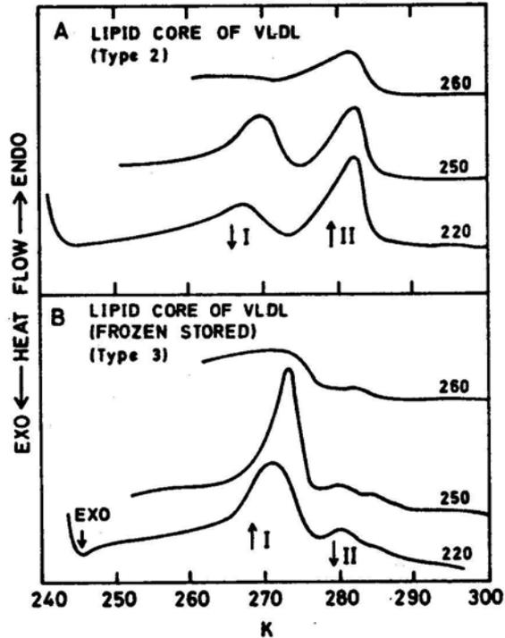
**Figure 3.** A. D.s.c. heating curves of a protease-treated 'lipid-core' of EYP containing 33% glycol. B. Transition curves of protease-treated 'lipid-core' of EYP stored frozen at  $-25^{\circ}\text{C}$  for 2 days before addition of glycol (33% final conc). Other details as in figure 1.
