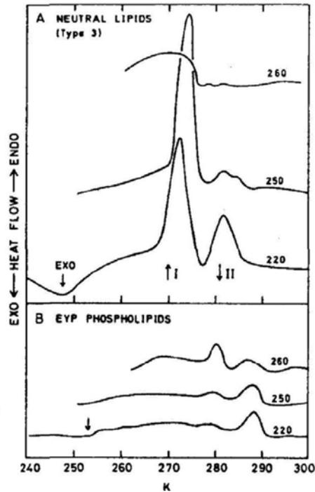
**Figure 2.** A. D.s.c. heating curves of neutral EYP lipids (triglycerides) in the neat form. B. Transitions of phospholipid fraction of EYP dispersed in water and containing 33% glycol. Other details as in figure 1.
