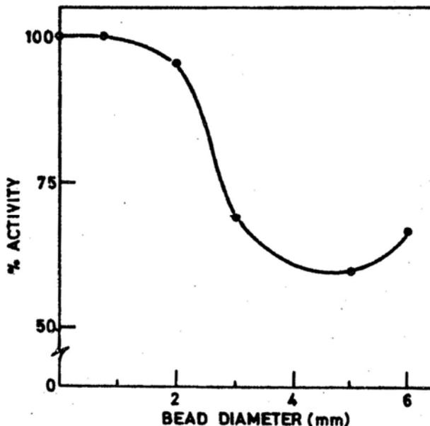
**Figure 1.** Effect of bead diameter on D-amino acid oxidase activity of immobilized *T. variabilis*.
