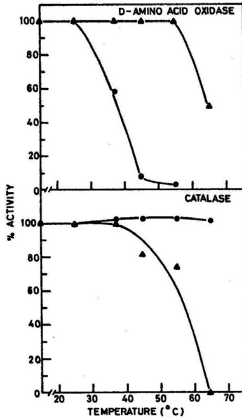
**Figure 4.** Thermostability of D-amino acid oxidase and catalase. The cell suspension was subjected to the desired temperature for 20 min and 10 min for D-amino acid oxidase and catalase respectively followed by rapid cooling by immersion in ice. Residual enzyme activity was determined. (●), Free cells; (▲), immobilized cells.
