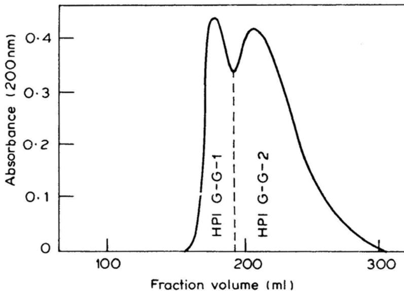
**Figure 3.** Elution profile of rechromatography of fraction HPI-G-100-2 on Sephadex G-100 column (3 × 150 cm). The elution buffer was 0.01 M sodium phosphate buffer, pH 7.4, the flow rate was 20 ml/h and the fraction volume was 5 ml.
