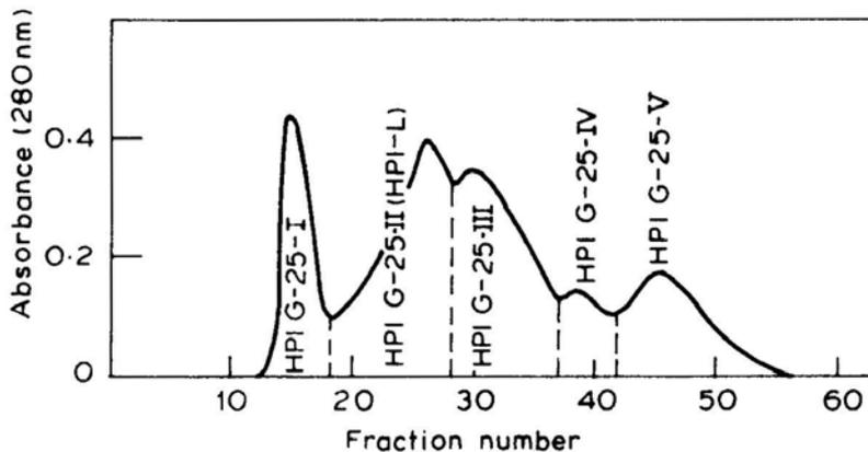
**Figure 2.** Elution profile of rechromatography of fraction HPI-G-100-3 on Sephadex G-25 column (2.5 × 40 cm). The elution buffer was 0.01 M sodium phosphate buffer, pH 7.4, the flow rate was 18 ml/h and the fraction volume was 3 ml.
