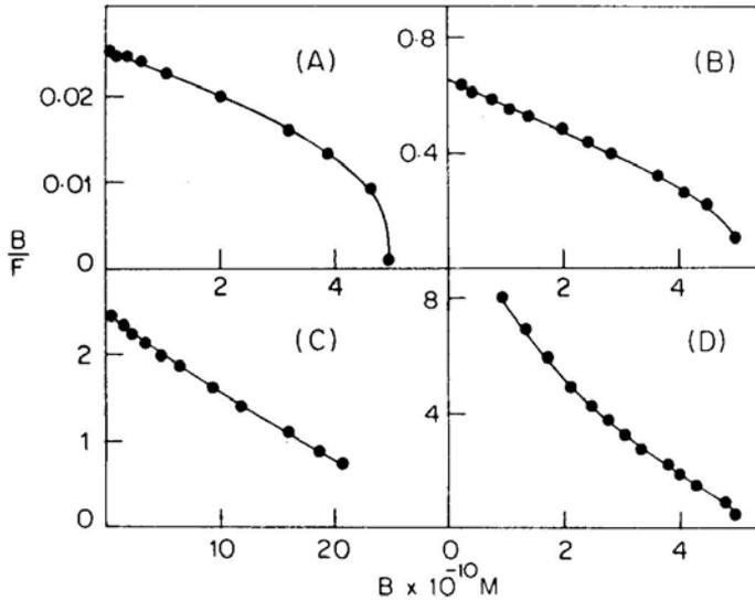
**Figure 4.** Theoretical Scatchard plots for irreversible systems. (A),  $a = 5 \times 10^{-10}$  M,  $k = 5 \times 10^6$ /h, and  $t = 10$ h. (B),  $a = 5 \times 10^{-10}$  M,  $k = 5 \times 10^8$ /h, and  $t = 10$ h. (C),  $a = 25 \times 10^{-10}$  M,  $k = 5 \times 10^7$ /h, and  $t = 10$ h. (D),  $a = 5 \times 10^{-10}$  M,  $k = 5 \times 10^8$ /h, and  $t = 10$ h.
