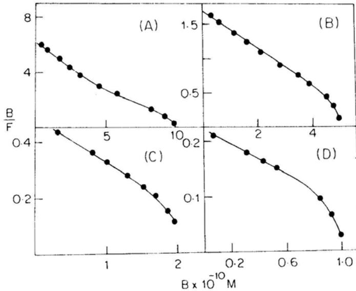
**Figure 7.** Plots are similar to those shown in figure 2 but in this case  $a$  is varied. Other variables were  $k = 2 \times 10^8/\text{h}$  and  $t = 10$  h. (A), (B), (C) and (D) correspond to a value of (receptor concentration)  $10 \times 10^{-10}$  M,  $5 \times 10^{-10}$  M,  $2 \times 10^{-10}$  M and  $1 \times 10^{-10}$  M respectively.
