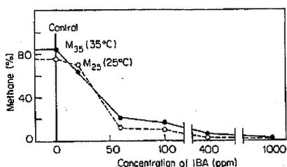
**Figure 2.** Inhibition of methane formation by IBA in M-25 and M-35 grown on acetate. Total incubation time - 2 days. Temperature of incubation was 25°C for M-25 and 35°C for M-35. Average concentration of IBA in a digester operating at ambient temperature varies between 40-60 ppm.
