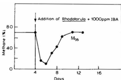
**Figure 3.** Reversal of inhibition of methane production by IBA using yeast *Rhodotorula*. The culture M-35 was stabilised at 35°C on acetate as a carbon source for 4 days. The IBA (1000 ppm) was added along with the preadapted cells of *Rhodotorula*. Details of the Experiment are presented in the text.
