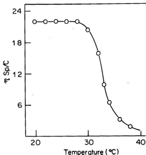
**Figure 1.** Denaturation curve of acid soluble collagen of skin of *Ophiocephalus* based on viscosity measurements at different temperatures.
